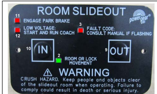
Figure 23 Touchpad. Reference of pins 2, 3, 9, 10, 11, and 12 from FIGURE 19 above
