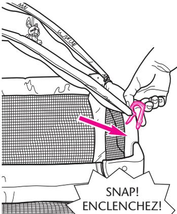
Snap plastic hooks on each end of the play gym onto the high arched sides of the play yard.
