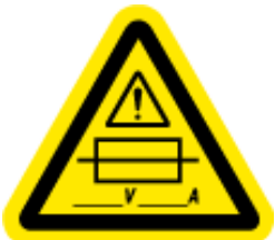
REPLACE FUSE WITH ONE OF PROPER RATING
