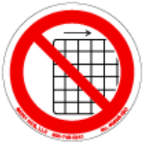
DO NOT OPERATE WITHOUT GUARDS IN PLACE
