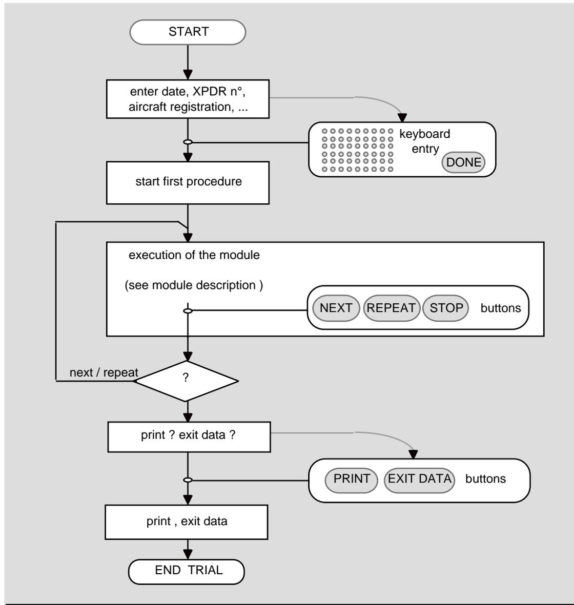
Figure 3 : 1 module for 1 trial ( a series of procedures ) / basic schematics
