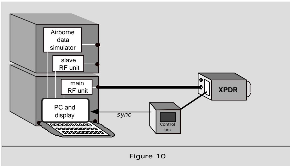
Test procedures P 6, P15, P16, P18, P21 to P28 use the following installation :
