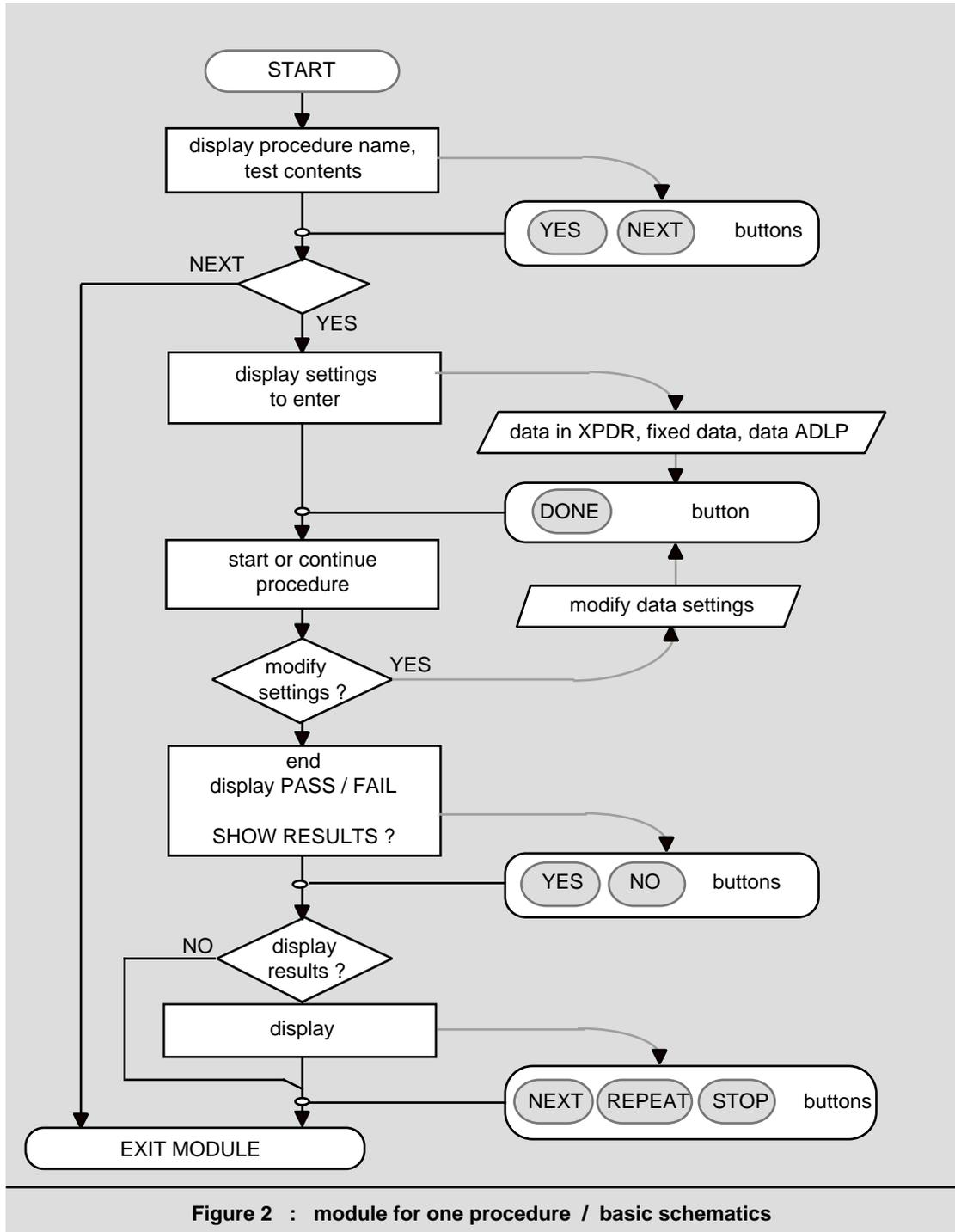
Figure 2 : module for one procedure / basic schematics
