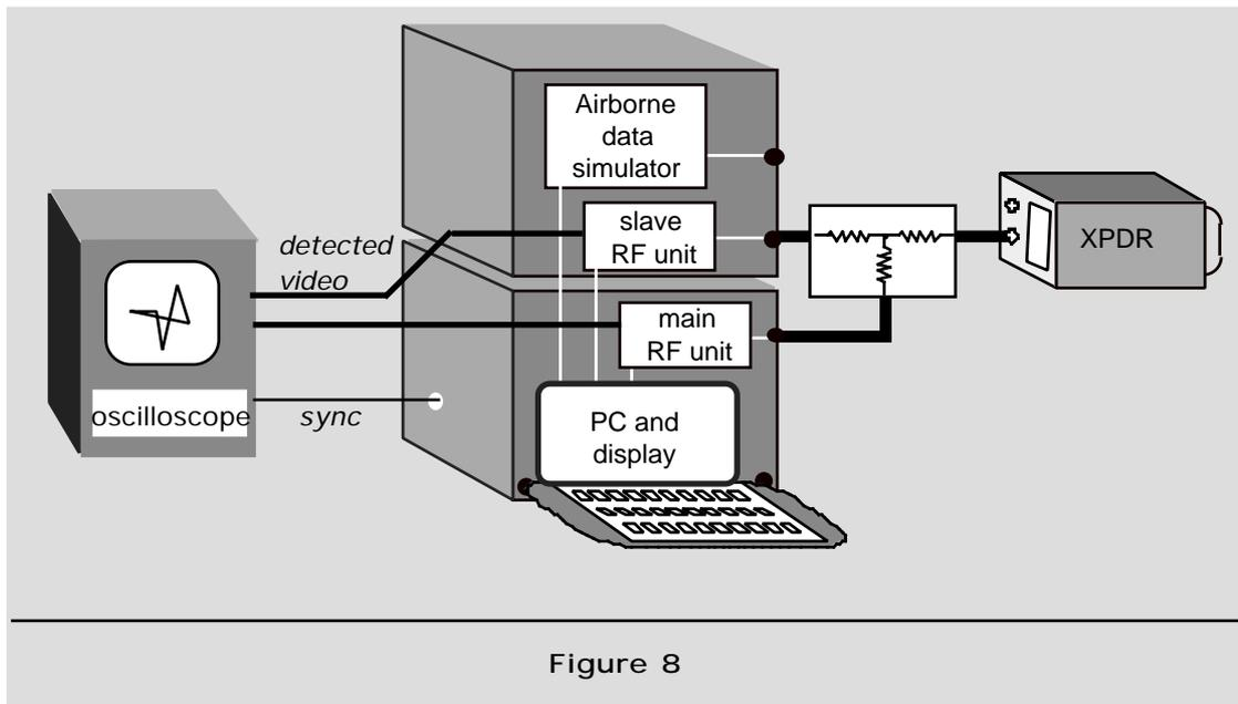
Test procedures P 76 uses the following installation :
