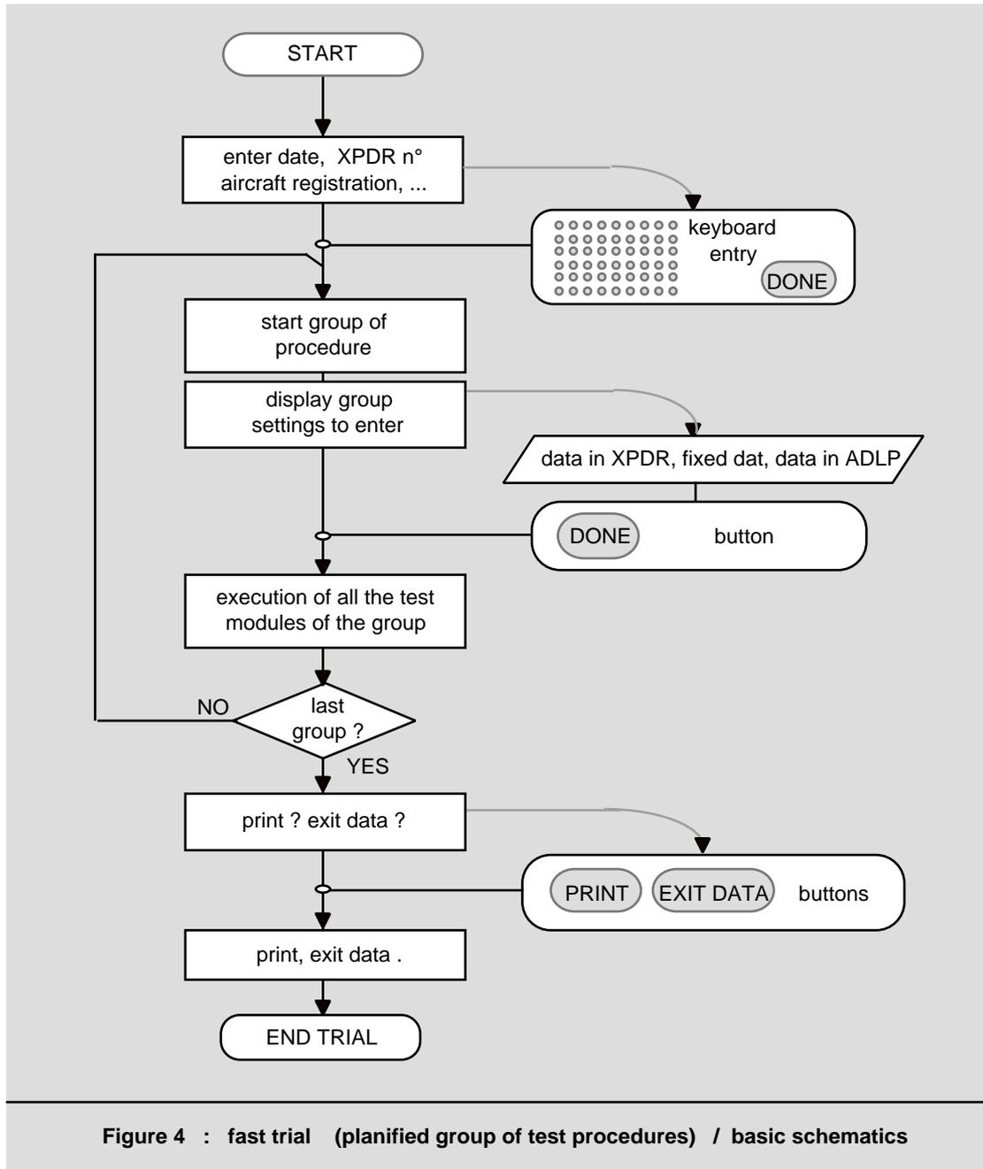
Figure 4 : fast trial (planned group of test procedures) / basic schematics
