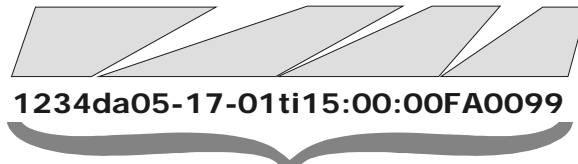
Figure 3-10: SIA DCS Coded Message Example for Fire Alarm Event.
