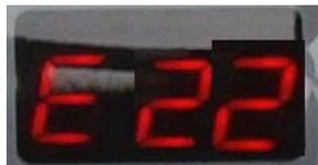
Error message: The memory function is failure
