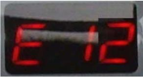
Error message: Drainage error, water not emptied within 5 min.
