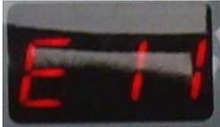
Error message: The required water level is not reached within 8 min
