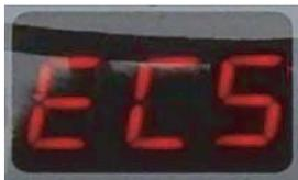
Error message: The dry temperature sensor short cut or open.
