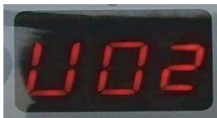
Error message: Door is not properly shut 20s after program is started.
