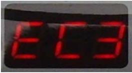
Error message: The water level sensor circuit short cut or open
