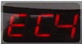
Error message: The temperature of air vent
