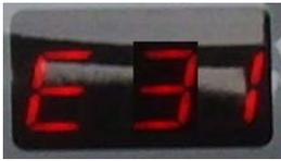
Error message. Motor overheat protection or is damaged.
