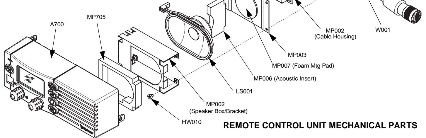
**REMOTE CONTROL UNIT MECHANICAL PARTS**
