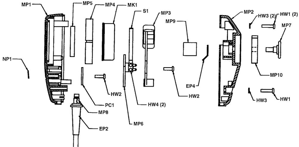
**AMPLIFIED DYNAMIC MICROPHONE SCHEMATIC AND MECHANICAL PARTS**
