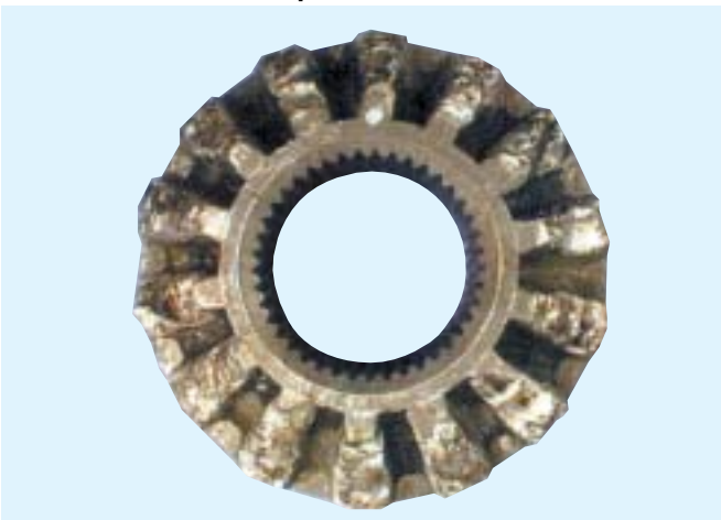
Side Gear - Catastrophic Shock
