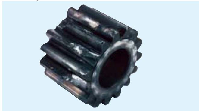
Planetary Gear - Shock Failure
