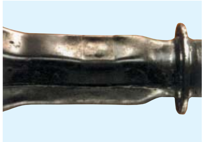
Over-torqued Clamping Hardware
