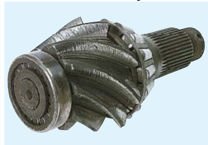
Drive Pinion - Low Lube - Scoring
