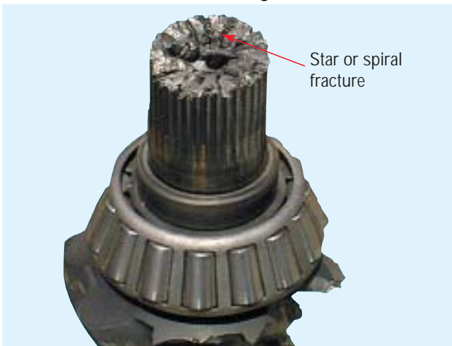
Drive Pinion - Torsional Fatigue Failure
