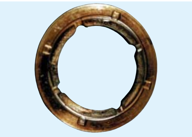
Power Divider Thrust Washer - Lubricant Contamination
