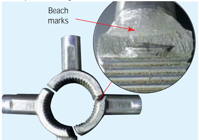
IAD Spider - Fatigue Failure
