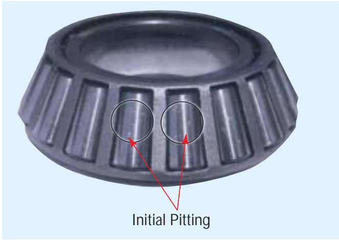
Bearing Cone - Spalling
