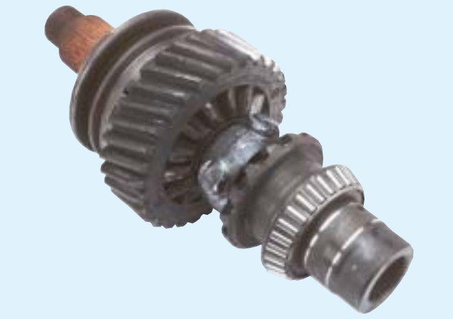
Helical Side Gear - Bushing Burn-Up
