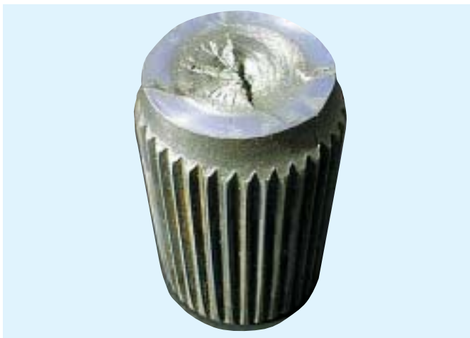
Axle Shaft - Torsional Fatigue Failure
