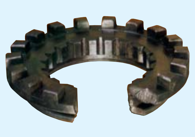
Sliding Clutch - Shock Failure
