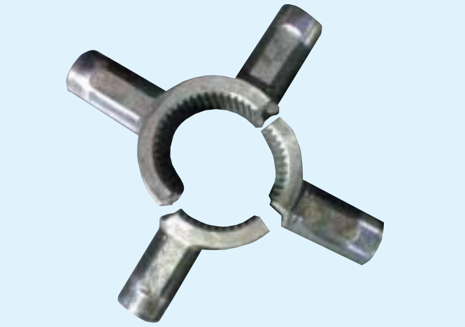
Sliding Clutch - Shock Failure
