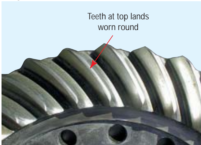
Ring Gear - Low Lube - Crows Foot
