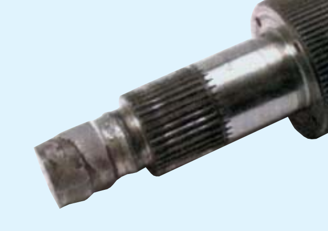
Output Side Gear - Stub-End Bore Galling
