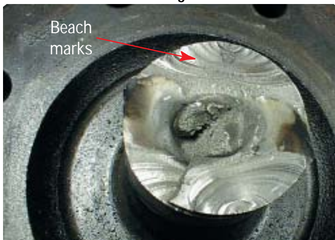
Axle Shaft - Torsional Fatigue Failure
