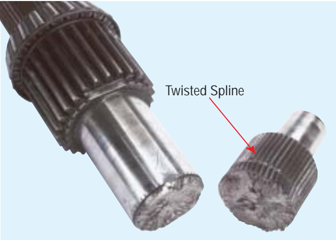
Input Shaft - Torsional Shock Failure
