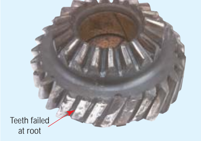
Input Shaft - Torsional Shock Failure
