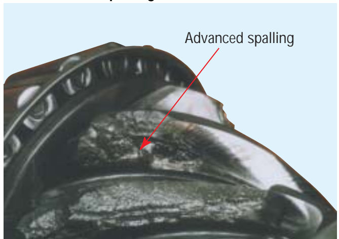
Drive Pinion - Spalling
