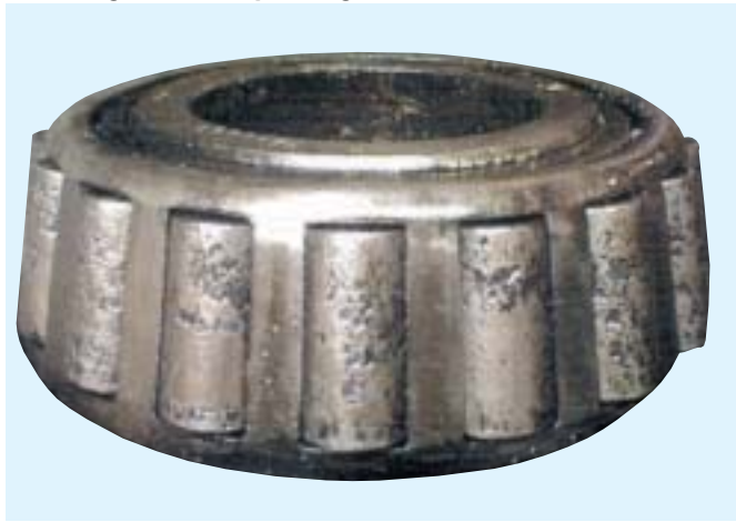
Bearing Cone - Spalling
