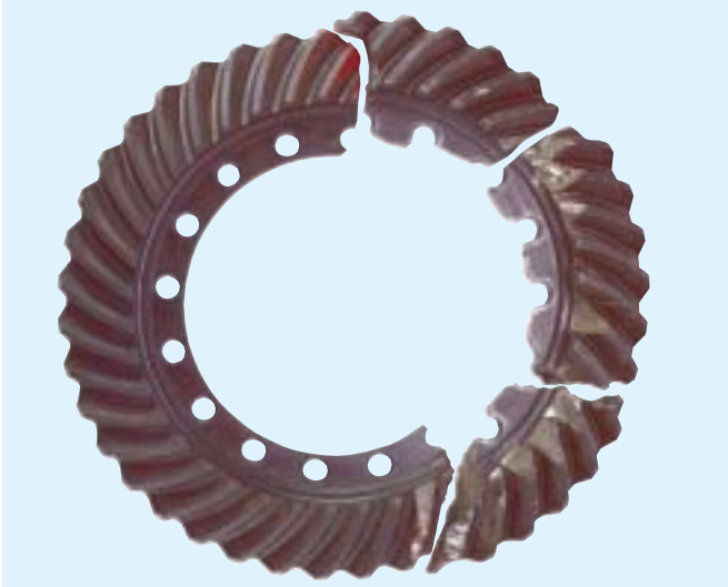
Drive Pinion - Torsional Shock Failure
