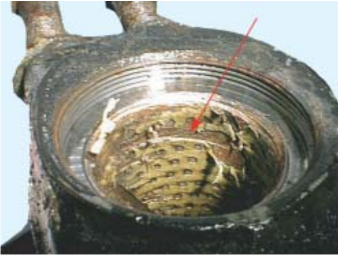
Improper Kingpin Installation
