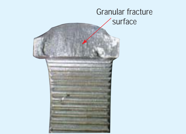
Side Pinion Gear - Shock Failure
