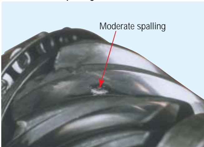
Drive Pinion - Spalling
