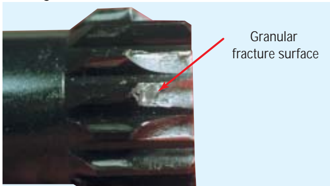
Sliding Clutch - Shock Failure
