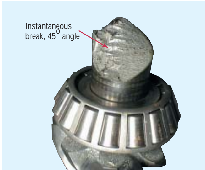
Drive Pinion - Torsional Shock Failure
