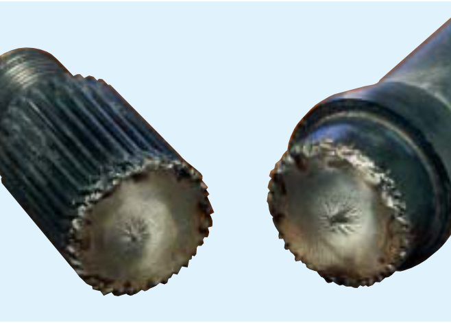
Output Shaft - Torsional Shock Failure
