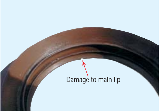
Damaged Seal Lip
