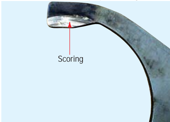
Power Divider Thrust Washer - Lubricant Contamination
