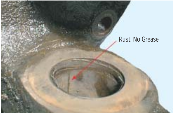
Bushing - Lack of Grease
