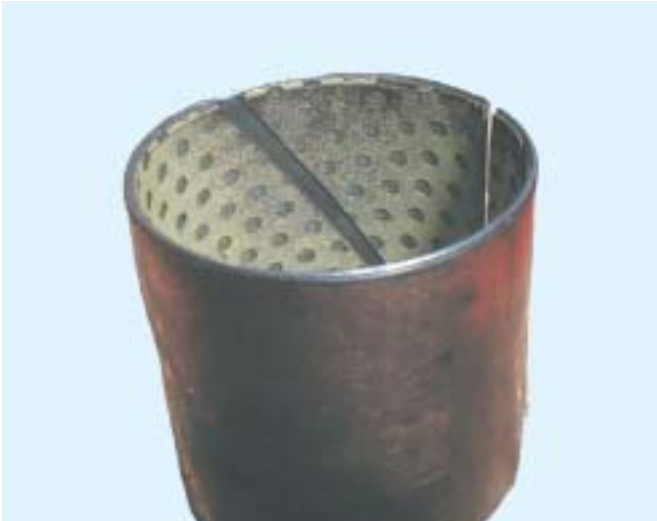
Bushing Worn in One Area Only
