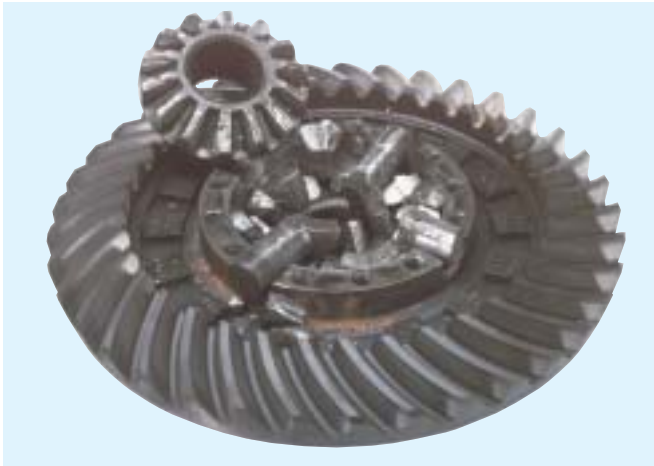
Side Gear - Catastrophic Shock
