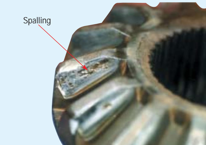
Output Side Gear - Spalling
