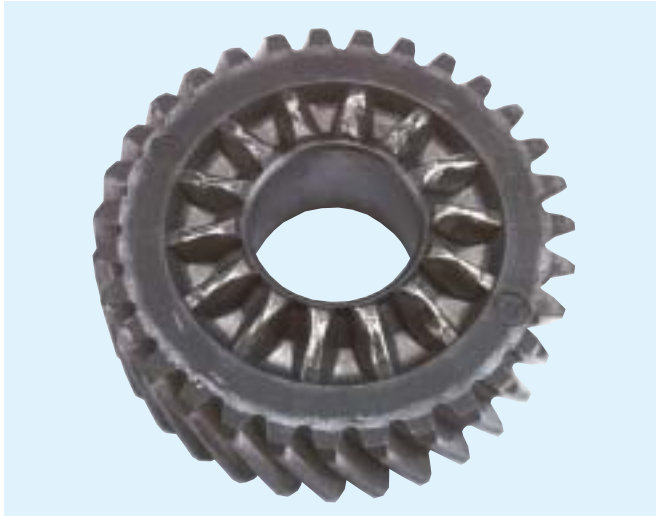
Helical Side Gear - Bushing Burn-Up
