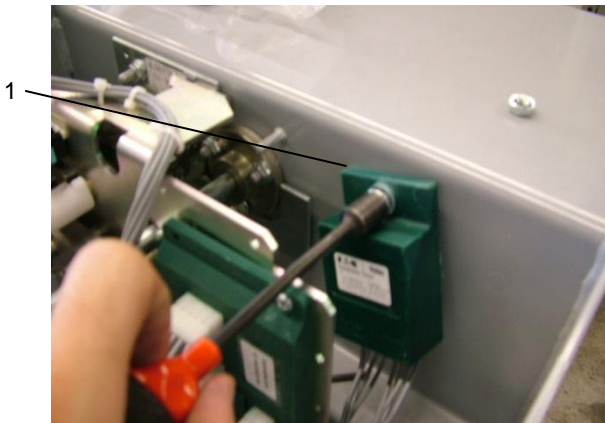
For transformer panel, place timer as shown, use the M6 flange nut with a 8 mm washer to secure it (1)
