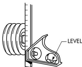
DO NOT over tighten belts or chains. Adjust chains to manufacturer's specifications. Adjust belts as follows: The ideal tension is the lowest tension at which the belt will not slip under peak load conditions. Check the belt tension frequently during the first 24 to 48 hours of run-in operation. Over tightening belts shortens belt and bearing life. Keep belts free from foreign material which may cause slippage. Inspect the V-belts periodically; tighten the belts if they are slipping.
