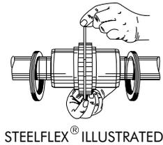
**OFFSET ALIGNMENT** — Align driving and driven shafts so that a straight edge will rest squarely on both coupling hubs as shown to the right and also at 90° intervals. Tighten foundation bolts of the connected equipment and recheck alignment and gap.
