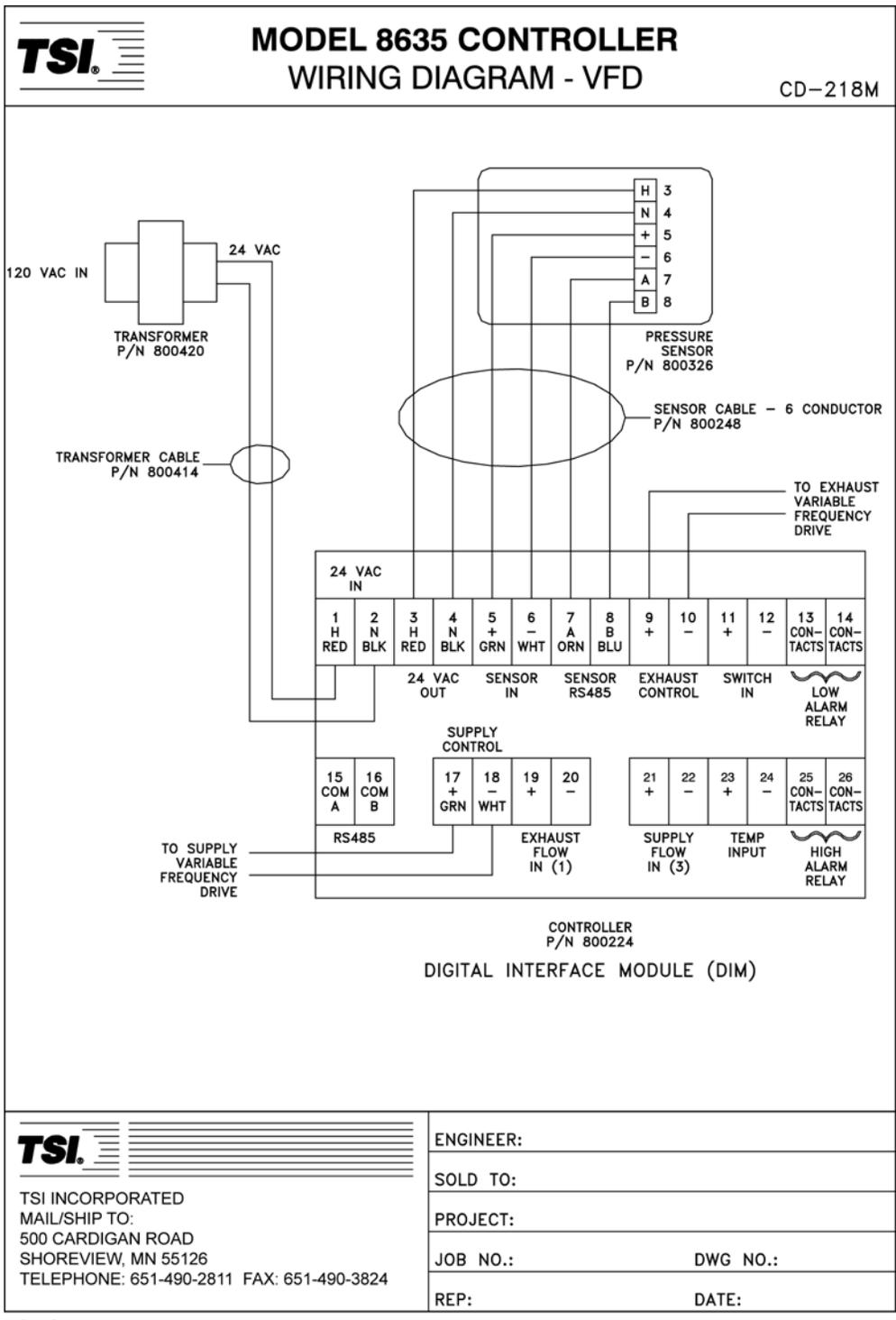
**Figure 12: Wiring Diagram - VFD Systems**
