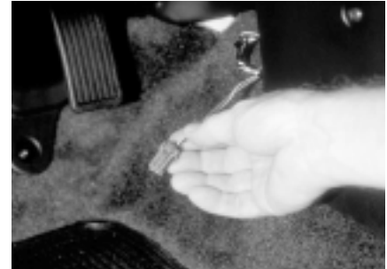
P13-3 Lower the vehicle and locate the service check connector behind the center console.
