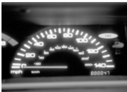
P13-7 Observe the 4WS indicator light flashes to obtain the fault codes.
