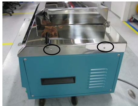
3. Loose 2 of screw at the right part.
