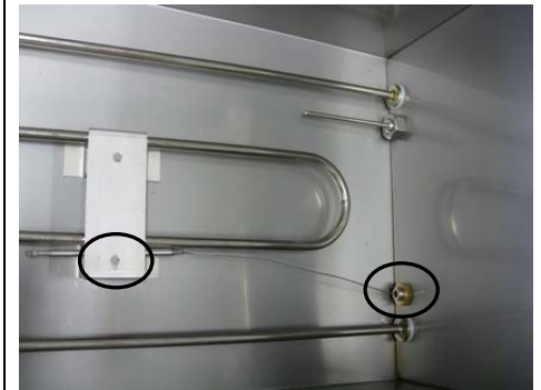
8. Temperature regulator can be separated when nut and screws are loosened..
