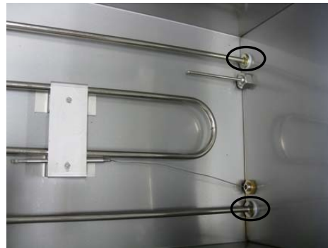
6. Heater can be separated to take out only nut 2 of nut.
