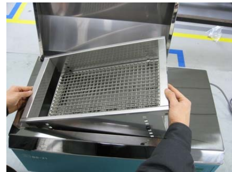
1. Separate tray. Refer to 2-1-6. Spring wire rack disassemble”
