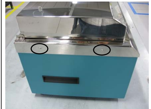
4. Loose 2 of screw at the left side. - Housing cover ≡ can be separated..
