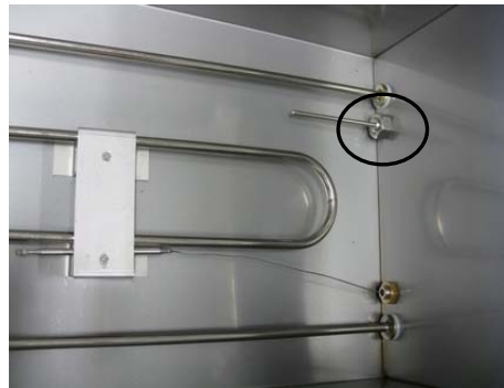
7. Temp.sensor can be separated when nut is loosen.
