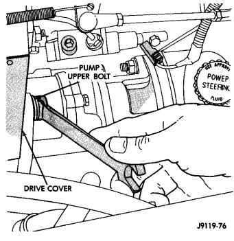
Fig. 7 Removing Pump Assembly Upper Mounting Bolt
