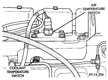
Fig. 3 Coolant Temperature Switch
