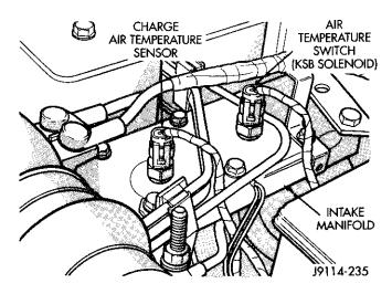
Fig. 7 Charge Air Temperature Sensor and Air Temperature Switch
