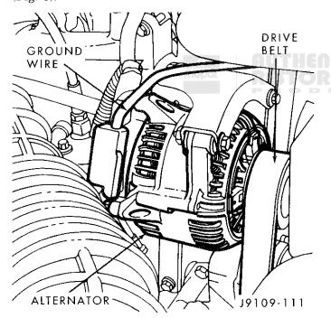
Fig. 5 Alternator Removal
