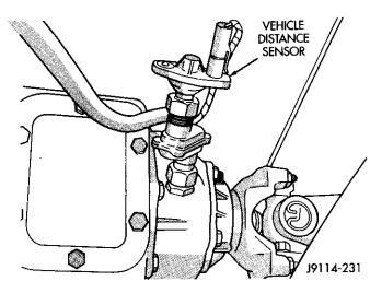
Fig. 6 Vehicle Distance Sensor
