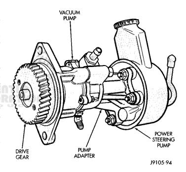
Fig. 1 Vacuum And Steering Pump Assembly
