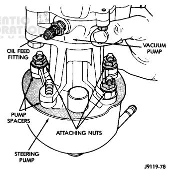
Fig. 6 Bracket Nut Removal/Installation
