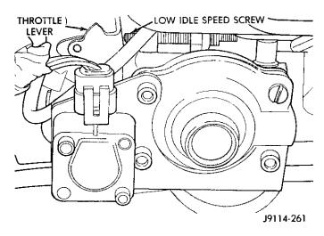
Fig. 3 Throttle Lever Contacting Low Idle Speed Screw
