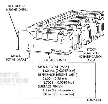
Fig. 10 Cylinder Head Stock Removal
