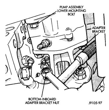
Fig. 6 Adapter And Pump Mounting Fastener
