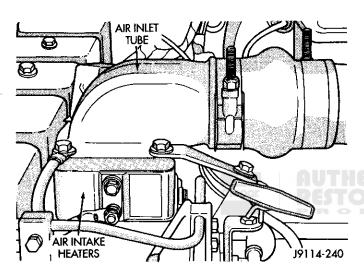
Fig. 4 Air Intake Heaters
