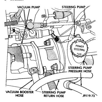
Fig. 1 Vacuum/Steering Pump Assembly
