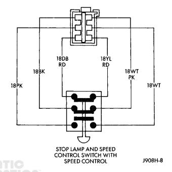
Fig. 5 Stop Lamp Switch Connector
