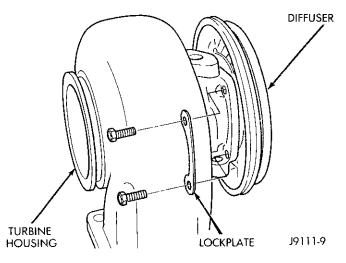
Fig. 12 Diffuser and Lockplate
