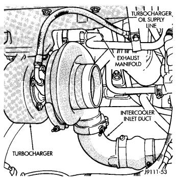
Fig. 2 Oil Supply Line and Intercooler Inlet Duct
