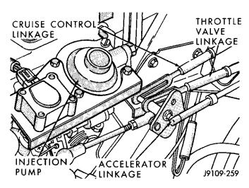
Fig. 6 Accelerator/Speed Control/Throttle Valve Linkage
