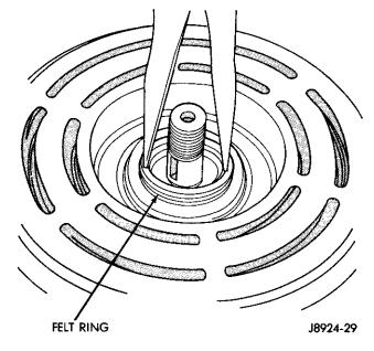
Fig. 14 Remove Felt Ring
