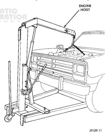
Fig. 11 Lifting Engine from Vehicle
