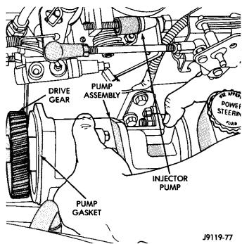
Fig. 5 Pump Assembly Removal/Installation
