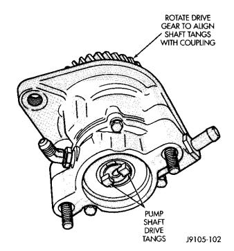
Fig. 10 Aligning Pump Shaft Drive Tangs
