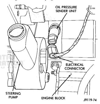
Fig. 2 Oil Pressure Sending Unit
