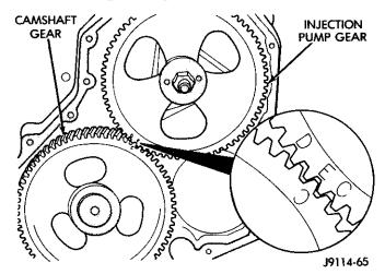
Fig. 22 Injection Pump to Engine Timing
