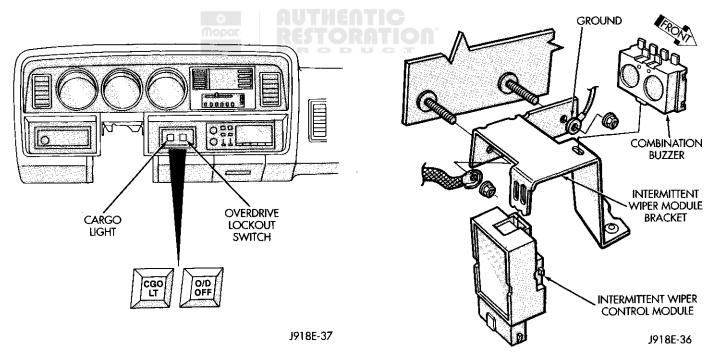
Fig. 1 Overdrive Lockout Switch Location
