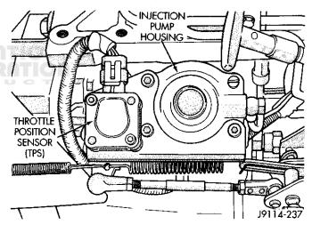
Fig. 5 Throttle Position Sensor
