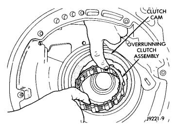
Fig. 3 Removing/Installing Overrunning Clutch
