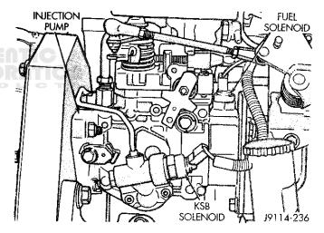
Fig. 6 KSB Solenoid Removal/Installation
