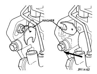
Fig. 18 Installing Lockscrew Washer
