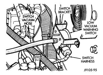
Fig. 2 Vacuum Switch Location
