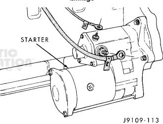
Fig. 7 Starter Connections
