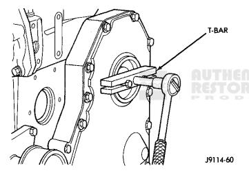
Fig. 16 Separating Pump Gear from Injection Pump Shaft
