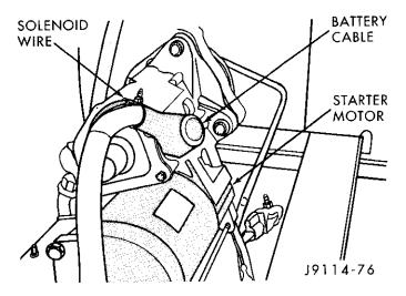
Fig. 4 Starter Motor Connections
