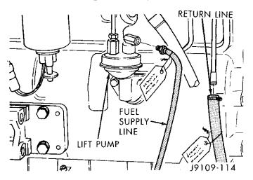
Fig. 9 Lift Pump and Fuel Lines
