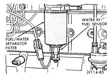
Fig. 6 Water-in-Fuel (WIF) Sensor
