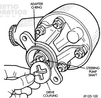
Fig. 11 Removing/Installing Pump Drive Coupling
