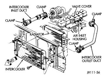
Fig. 4 Intercooler Ducts
