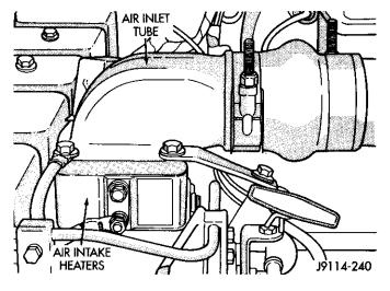
Fig. 9 Air Intake Heaters
