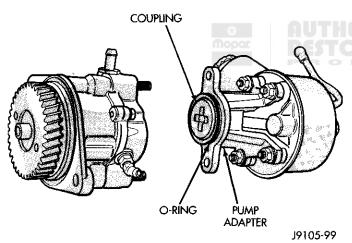
Fig. 9 Vacuum Pump Removed From Adapter
