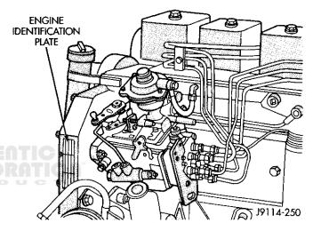
Fig. 19 Engine Identification Plate
