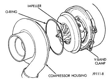
Fig. 11 Compressor Housing and Impeller
