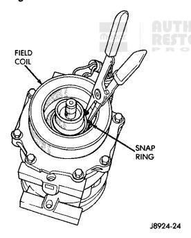
Fig. 9 Remove Snap Ring and Field Coil
