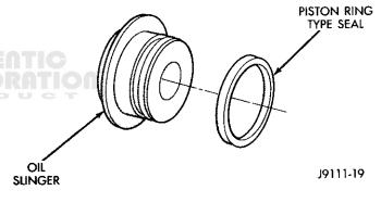
Fig. 22 Piston Ring Type Seal
