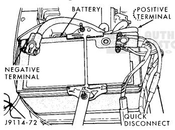
Fig. 1 Battery Connections
