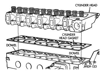
Fig. 11 Cylinder Head/Gasket Alignment
