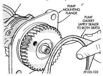
Fig. 13 Positioning Gasket On Pump Mounting Flange
