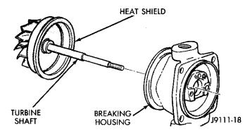
Fig. 19 Turbine Shaft/Heat Shield to Bearing Housing
