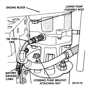
Fig. 3 Oil Feed Line Removal/Installation
