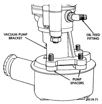
Fig. 8 Steering/Vacuum Pump Assembly
