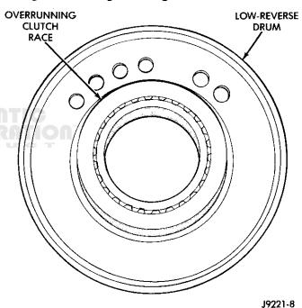
Fig. 2 Overrunning Clutch Race Position
