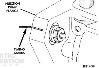
Fig. 14 Injection Pump Timing Marks
