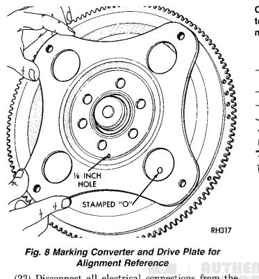
Fig. 8 Marking Converter and Drive Plate for Alignment Reference
