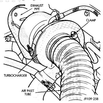
Fig. 3 Air Inlet Tube and Exhaust Pipe Connection
