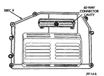
Fig. 1 Engine Controller
