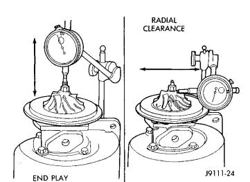
Fig. 28 End Play/Radial Clearance of Shaft
