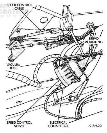
Fig. 1 Speed Control System
