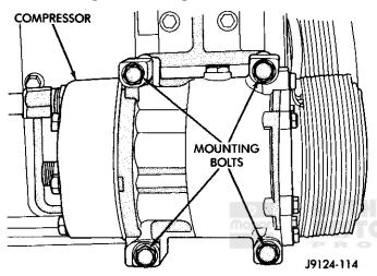
Fig. 1 Compressor Mounting (5.9L Diesel)
