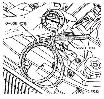
Fig. 6 Vacuum Gauge Test
