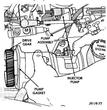
Fig. 14 Installing Pump Assembly On Engine
