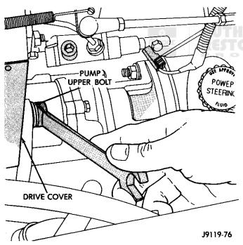
Fig. 4 Pump Assembly Upper Bolt
