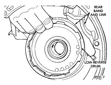
Fig. 1 Removing/Installing Low-Reverse Drum
