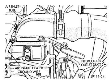
Fig. 5 Air Inlet Tube and Heater Ground Wire
