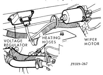
Fig. 10 Wiper Motor/Voltage Regulator
