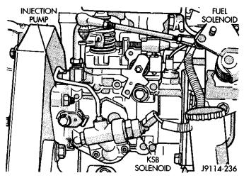
Fig. 7 Fuel Solenoid and KSB Solenoid
