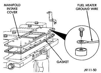
Fig. 8 Manifold Intake Cover and Fuel Heater Ground Wire
