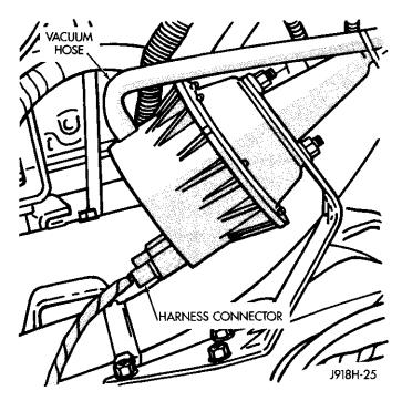
Fig. 2 Servo And Harness Connector
