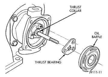
Fig. 14 Oil Baffle, Thrust Bearing and Collar
