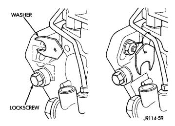
Fig. 15 Injection Pump Shaft LockScrew and Washer
