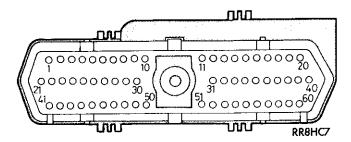
Fig. 4 Engine Controller 60-Way Connector Shown from Terminal End
