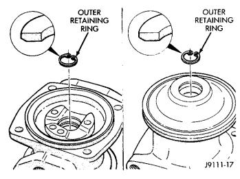
Fig. 21 Beveled Face of Outer Retainer Ring
