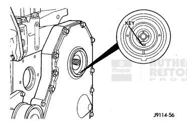
Fig. 12 Injection Pump Key-Way
