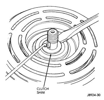
Fig. 15 Remove Clutch Shim
