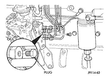
Fig. 20 Timing Indicator Plug
