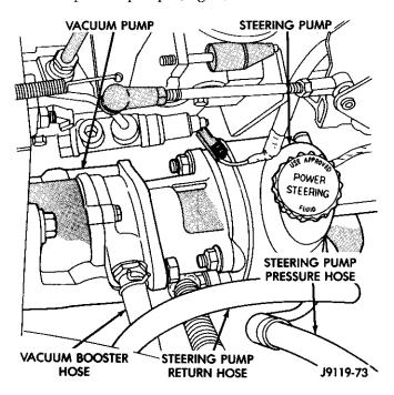
Fig. 3 Vacuum And Steering Pump Hose Connections
