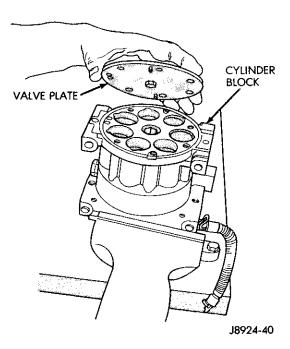
Fig. 24 Remove Valve Plate
