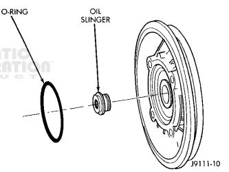
Fig. 13 Diffuser, O-Ring and Oil Slinger
