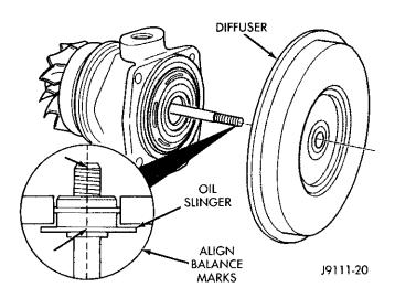
Fig. 23 Align Balance Marks-Shaft and Oil Slinger
