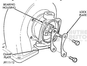
Fig. 15 Turbine Housing Lock Plates and Clamp Plates
