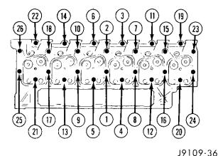
Fig. 7 Cylinder Head Bolt Removal Sequence—Cylinder Head Hot
