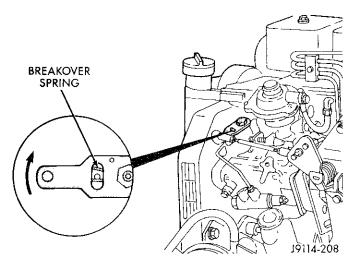
Fig. 5 Correct Breakover Spring Position
