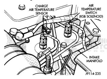
Fig. 11 Air Temperature Switch
