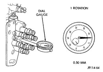
Fig. 21 Checking Injection Pump Timing
