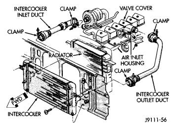
Fig. 30 Intercooler Ducts
