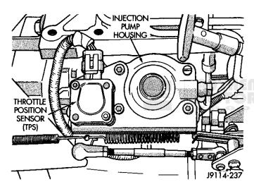
Fig. 1 Throttle Position Sensor
