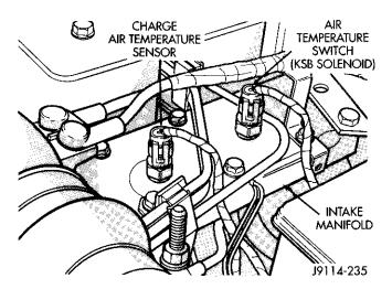
Fig. 2 Charge Air Temperature Sensor
