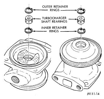
Fig. 17 Snap Rings and Shaft Bearing
