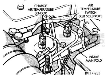
Fig. 5 Charge Air Temperature Sensor and Air Temperature Switch
