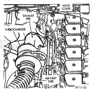
Fig. 9 Air Intake Pipe, Exhaust Pipe and Turbocharger
