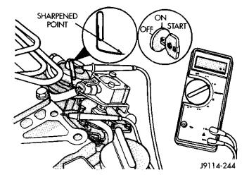
Fig. 13 Throttle Position Sensor (TPS) Testing
