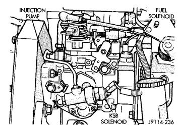
Fig. 10 KSB Solenoid Valve
