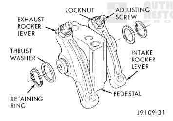
Fig. 2 Location of Rocker Lever Components
