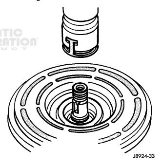
Fig. 18 Remove Seal Assembly
