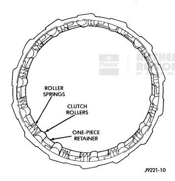
Fig. 4 Clutch Roller, Spring And Retainer Assembly
