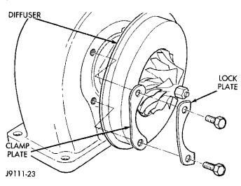
Fig. 26 Install Clamp Plates/Lock Plates
