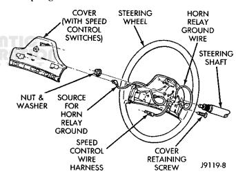
Fig. 1 Speed Control Switch Removal
