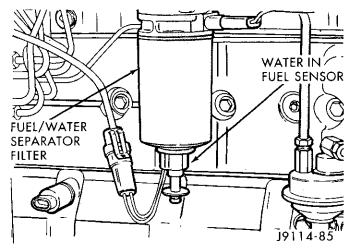
Fig. 6 Fuel/Water Separator Filter
