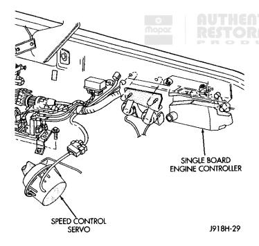
Fig. 3 Engine Controller and Connector Location
