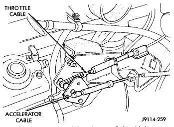
Fig. 9 Throttle and Accelerator Cable Linkage
