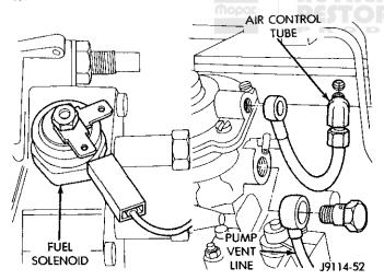
Fig. 8 Fuel Solenoid, Air Control Tube, Pump Vent Line
