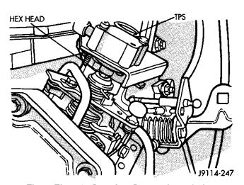
Fig. 2 Throttle Position Sensor Installation
