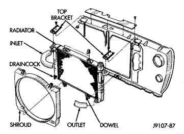
Fig. 1 Radiator and Fan Shroud
