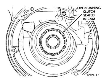
Fig. 5 Overrunning Clutch Seated In Cam
