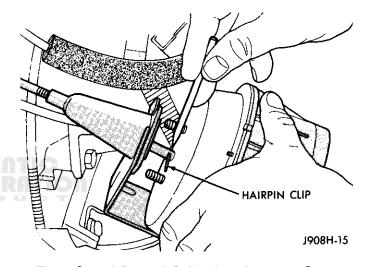
Fig. 7 Speed Control Cable Attachment at Servo
