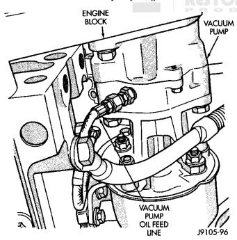
Fig. 5 Oil Feed Line Connection At Pump
