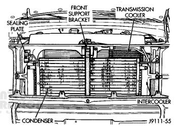
Fig. 29 Condenser and Intercooler
