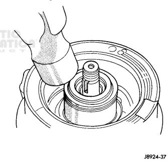
Fig. 20 Install Seal Assembly
