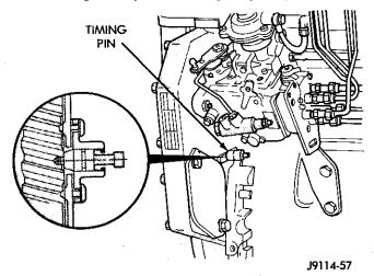
Fig. 13 Timing Pin-Cylinder No. 1
