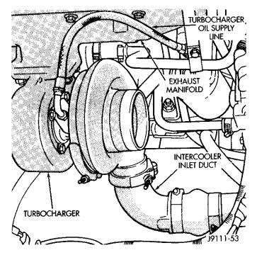
Fig. 10 Oil Supply Line and Intercooler Inlet Duct
