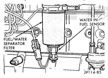
Fig. 7 Water-in-Fuel Sensor
