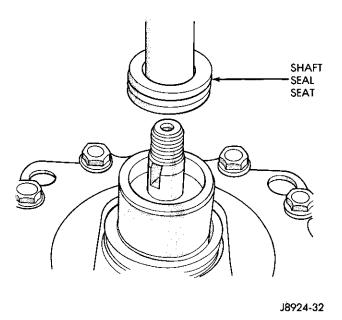
Fig. 17 Remove Shaft Seal Seat
