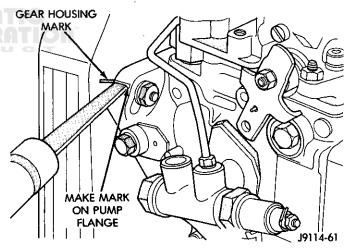
Fig. 17 Marking New or Rebuilt Injection Pump
