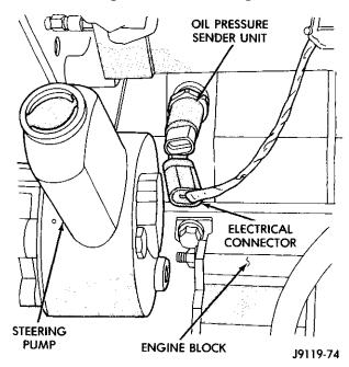
Fig. 4 Oil Pressure Sender Location
