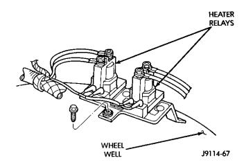
Fig. 8 Air Intake Heater Relays
