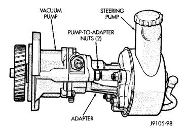
Fig. 8 Pump Assembly Removal
