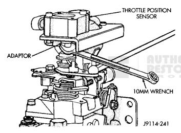
Fig. 4 Adjusting Throttle Position Sensor
