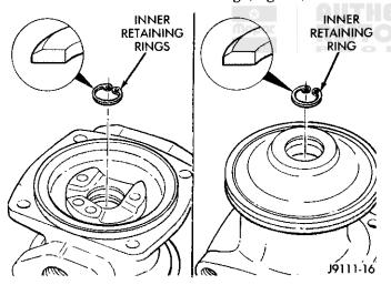
Fig. 20 Beveled Face of Inner Retainer Ring
