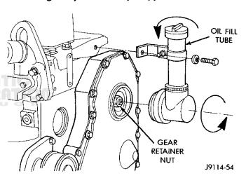
Fig. 10 Oil Fill Tube and Bracket
