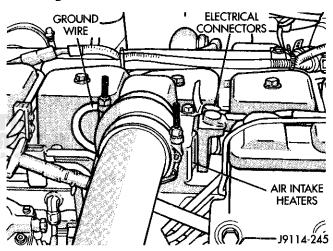
Fig. 8 Air Intake Heater
