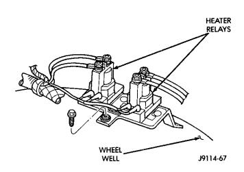
Fig. 3 Air Intake Heater Relays
