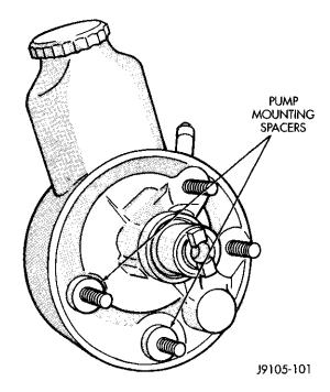
Fig. 12 Steering Pump Mounting Stud Spacer Locations
