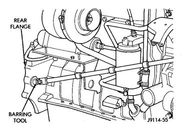
Fig. 11 Rotating Engine with Barring Tool
