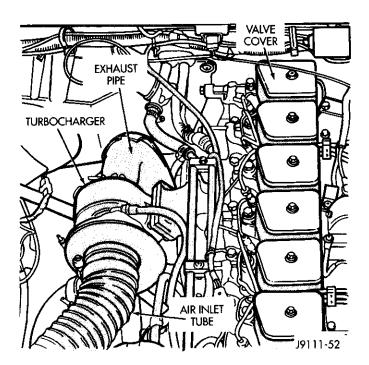
Fig. 1 Air Intake Pipe, Exhaust Pipe and Turbocharger
