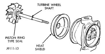
Fig. 16 Turbine Wheel Shaft and Heat Shield
