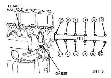
Fig. 4 Exhaust Manifold Bolt Tightening Sequence
