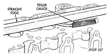
Fig. 9 Cylinder Head Combustion Deck Face Measurement
