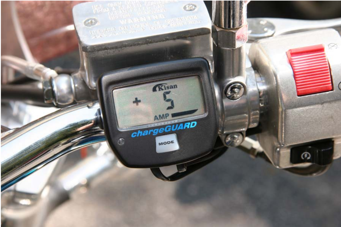
5 Amps of Charge Current Shortly After Starting Engine
