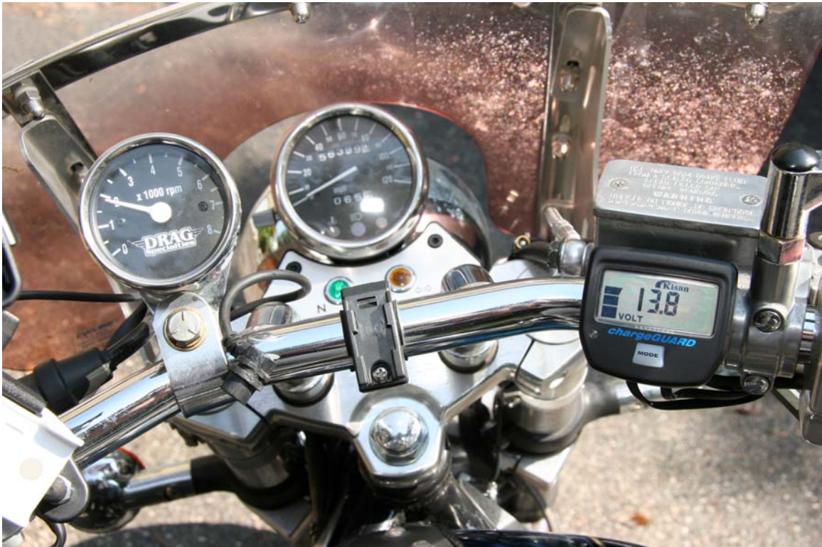
Charging System Voltage (13.8V) at 1800RPM
