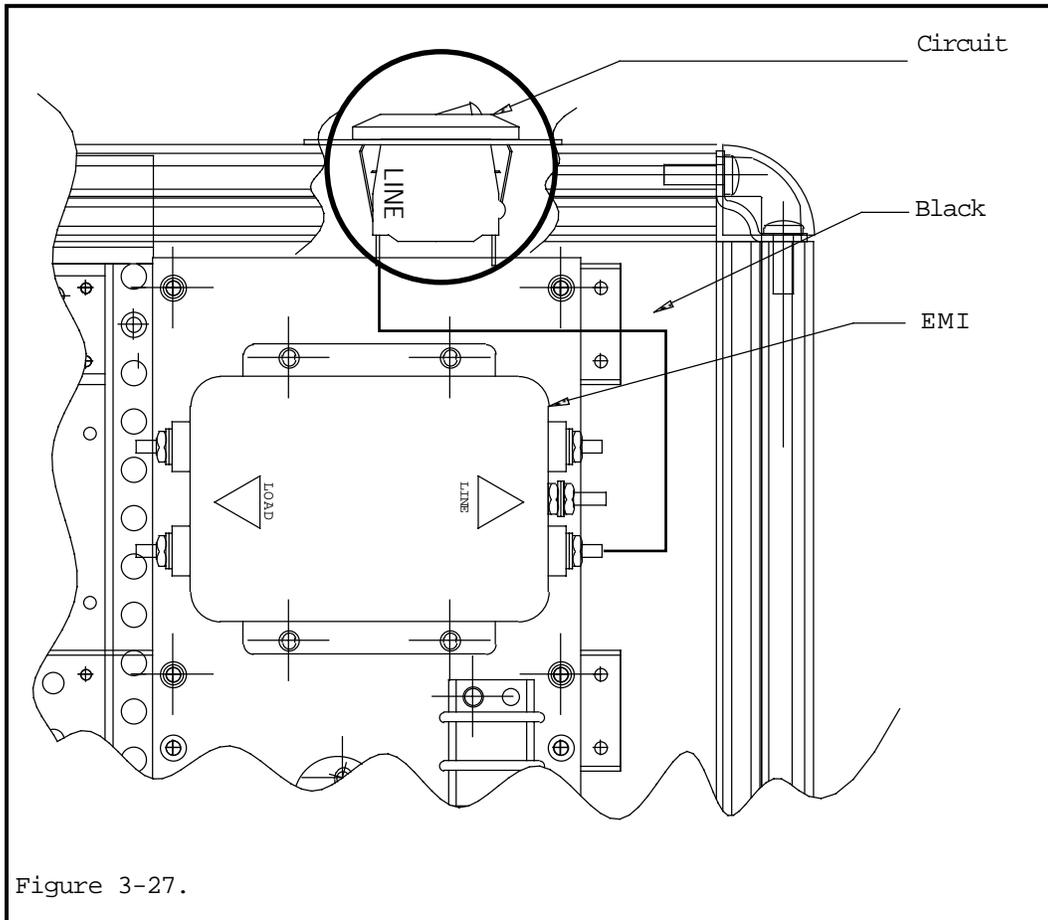
*Inserting Replacement Circuit Breaker*
