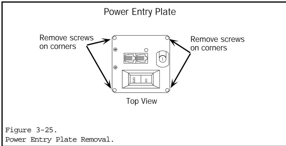
3. Use a screwdriver to remove the four screws which hold the power entry plate to the ALPHAVISION display.
