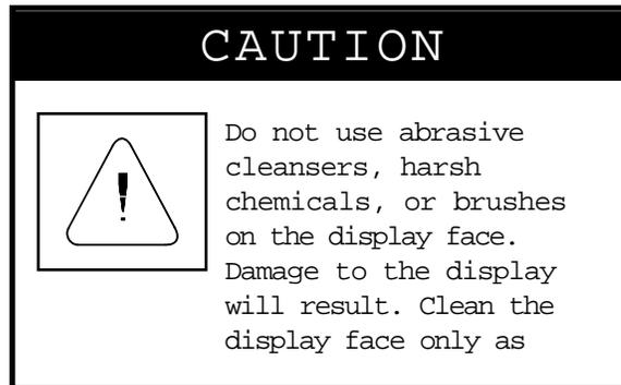
The front lens (the polycarbonate display face) will require occasional cleaning for best viewing. Adaptive Micro Systems recommends using a soft cloth and *Miller-Stephenson MS-260 Safezone Cleaner* (or another cleaner designed specifically for cleaning polycarbonate lenses.) A mild soap and water mixture may also be used.
