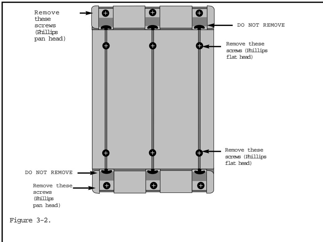
4. With the screws removed, lift the side panel up from the bottom (away from the display), then slide it towards the top of the display until it is completely removed.
