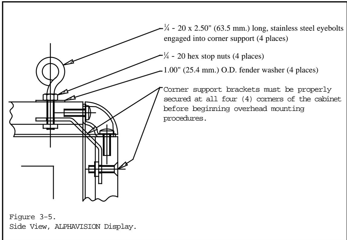
8. There must be a minimum of 1" (25.4 mm.) clearance on the top and the bottom of the ALPHAVISION display to allow for adequate ventilation. Without adequate ventilation, the ALPHAVISION can malfunction and become damaged.
