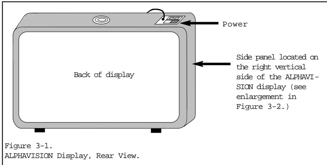
2. On a flat, level surface, place the ALPHAVISION display on its feet with the back of the display facing you. The fan and power switch should be facing up (see figure 3-1.)
