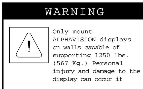
2. Mount the ALPHAVISION display on a sturdy wall. Adaptive Micro Systems highly recommends using a masonry wall. The wall bracket must be attached to a wall capable of supporting 1250 lbs. (567 Kg.)
