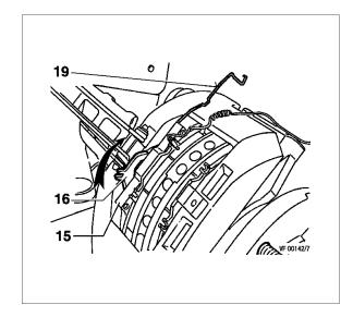
7.6 By displacing the Brake Caliper (1) toward the vehicle centre, the Thrust Plaste (15) can be pulled out of its location. After pulling out the inboard brake pad (12/1), the Caliper can be slid toward the road wheel, whereupon the outboard Brake Pad (12/2) can also be removed.
