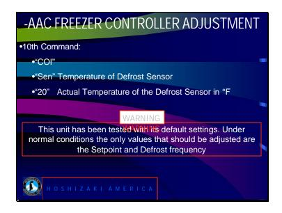
"COI" The next series of displays refer to temperature of the defrost Sensor.
