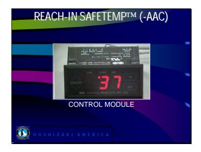
The –AAC uses a simple control module and two thermistors (Cabinet and defrost) to control the operation of the reach-in. A different controller is used for the Refrigerator and freezer. However the setpoint adjustment procedure is done the same on both controls
