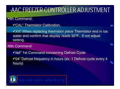
"CAL" Indicates the next display is for calibration of the thermistor.
