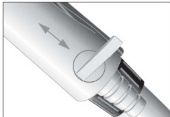
Figure 10: Fully Closed Resector Handpiece Suction Lever
