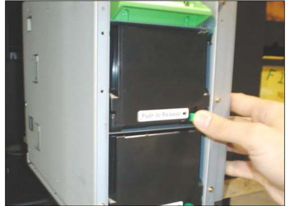
3. On the opposite side of the release button is another button that unlocks the top of the cartridge. Push it, and swing open the top.
