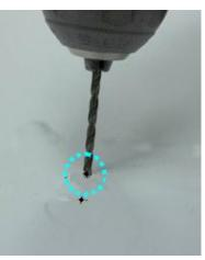
6. On the removed bumper, drill a 3mm pilot hole at the locations previously marked with the punch.
