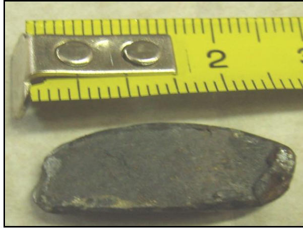
Photo No. 2: No. 2 Inlet valve segment
