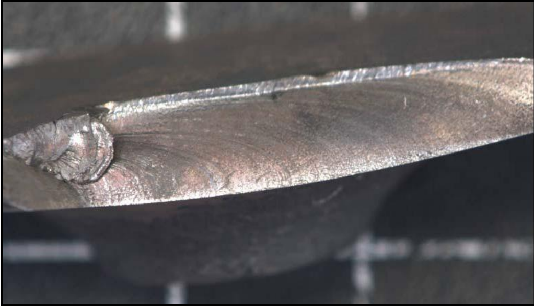
Photo No. 6: No. 2 Inlet valve fatigue crack (Engine Manufacturer's photo)
