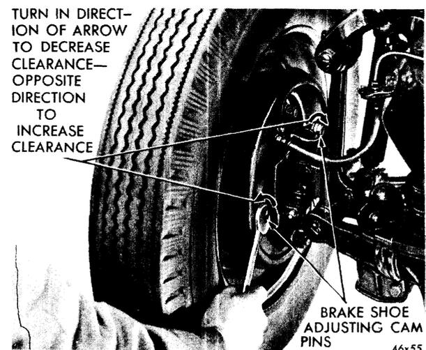
Fig. 11—Turning Brake Adjusting Cam (Typical View)
