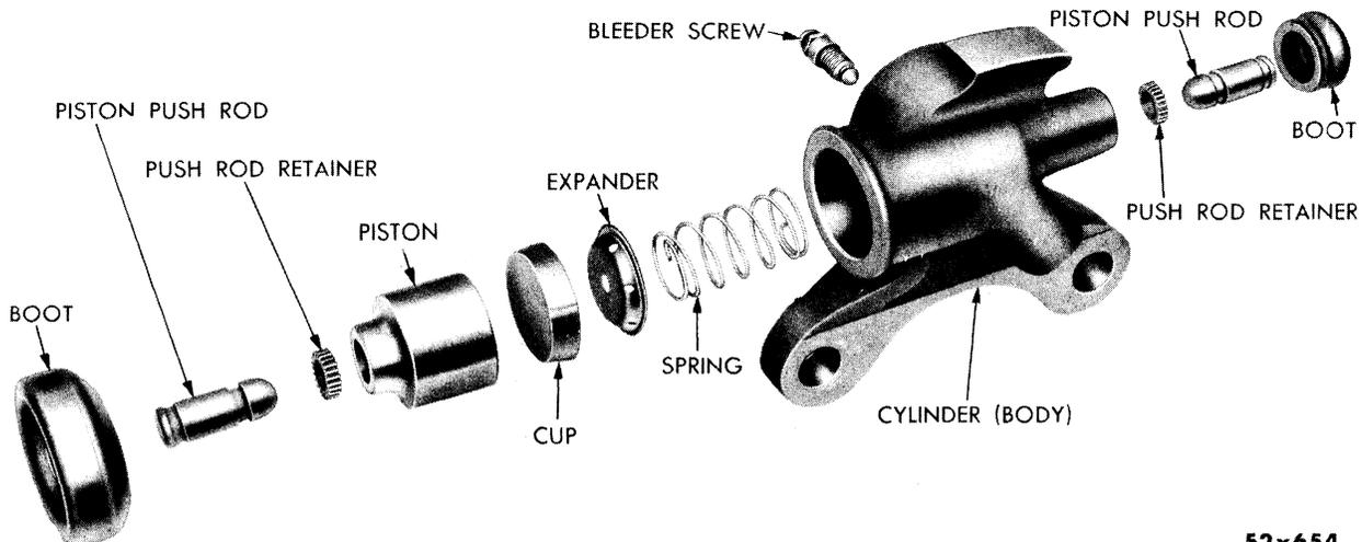
Fig. 40—Front Wheel Brake Cylinder (Disassembled View)
