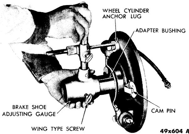
Fig. 16—Checking Height of Brake Shoe Adjusting Pin, Using Tool MT-19-L
