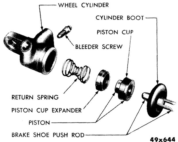
Fig. 7—Front Wheel Cylinder (Disassembled View)
