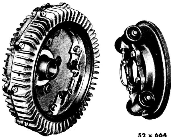
Fig. 53—Removing or Installing Rear Disc Brake Hub and Housing
