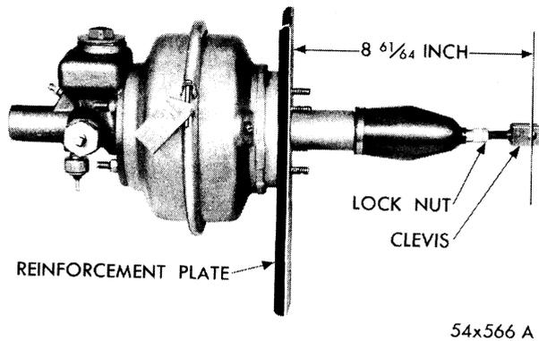
Fig. 89—Push Rod Adjustment (Unit Removed from Vehicle)
