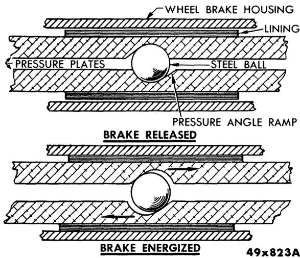
Fig. 39—Self-Energization Illustrated
