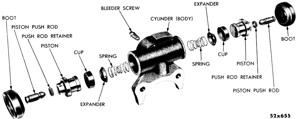
Fig. 41—Rear Wheel Brake Cylinder (Disassembled View)
