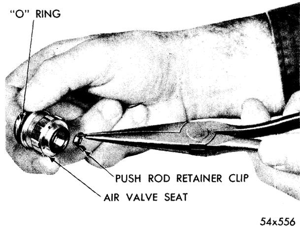
Fig. 79—Removing Push Rod Retainer Clip
