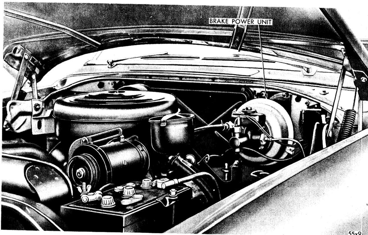
Fig. 90—Brake Power Unit Installed
