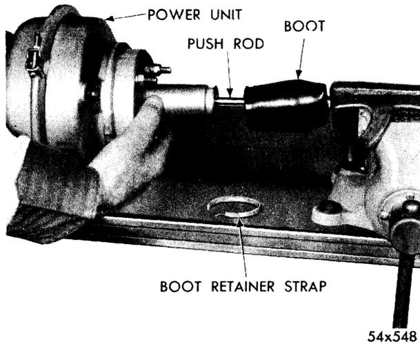
Fig. 71—Removing Push Rod from Unit
