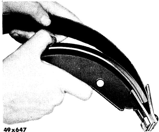
Fig. 31—Installing Shoe and Lining in Clamp
