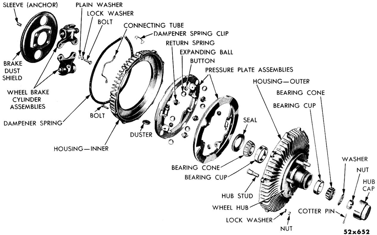
Fig. 36—Front Disc Brake (Disassembled View)
