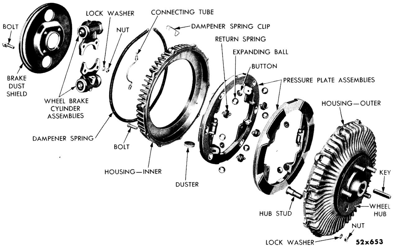
Fig. 37—Rear Disc Brake (Disassembled View)
