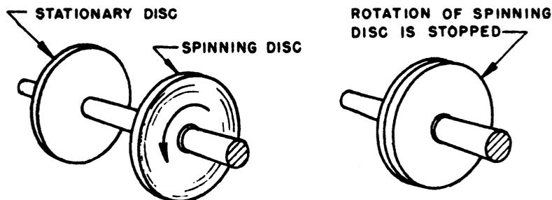
Fig. 38—Relation of Spinning and Stationary Discs
