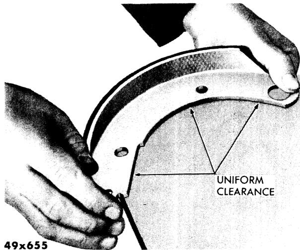
Fig. 15—Checking Shoe for Twist
