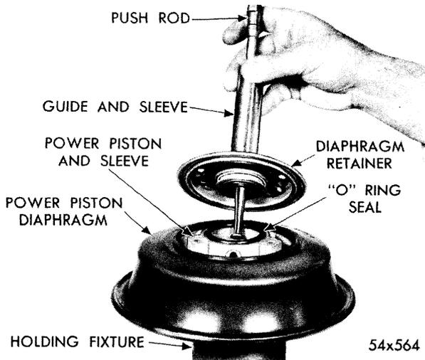
Fig. 87—Installing Guide and Sleeve to Power Piston
