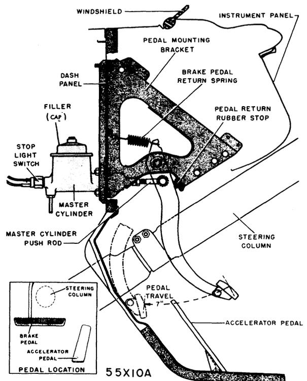
Fig. 3—Master Cylinder Location and Linkage
