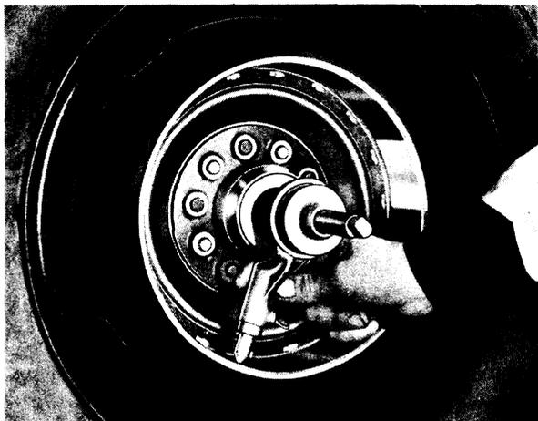
Fig. 19—Checking Brake Drum Diameter
