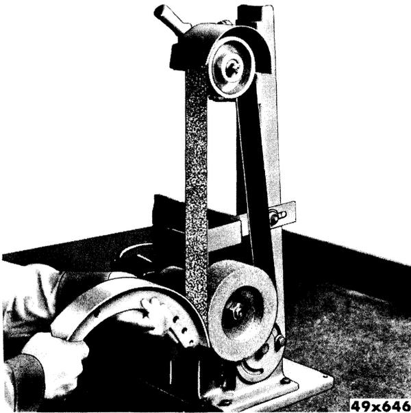
Fig. 29—Sanding Brake Shoe
