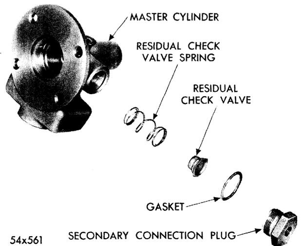
Fig. 84—Residual Check Valve (Disassembled View)
