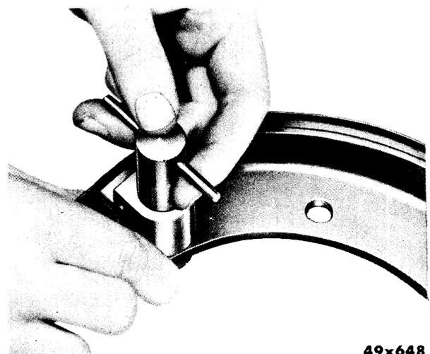
Fig. 32—Inserting Clamp Pin Anchor Hole
