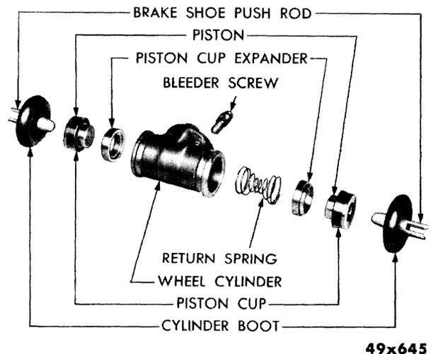
Fig. 8—Rear Wheel Cylinder (Disassembled View)
