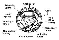
Typical drum brake components
