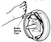
Using a brake spring tool to remove shoe return springs
