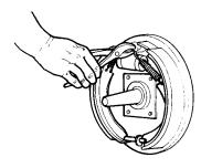
Installing hold-down spring pins
