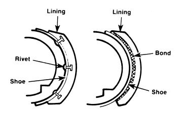
Riveted vs. bonded linings
