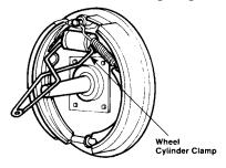
Clamping the wheel cylinder pistons
