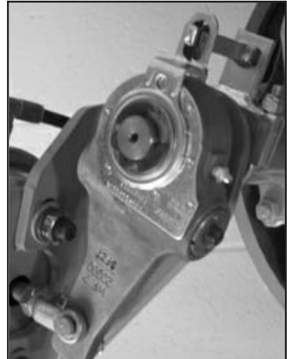
Figure 4 Mack drive axle with clamp bracket and flat anchor stud
