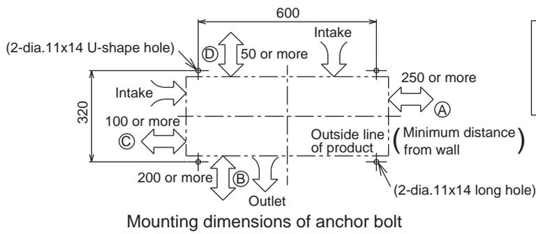
When installing the outdoor unit, leave open in at least two of directions (A),(B),(C)and(D) shown in the figure below.
