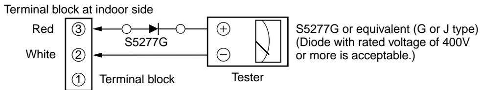
Normal time : Voltage swings between DC15 and 60V. ....Inverter Assembly check (11-8-1.)
