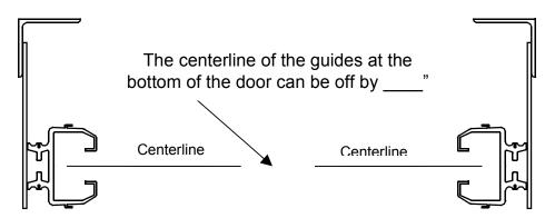
The guides are centered perfectly at the header box, and must be centered perfectly at the bottom. Make sure the guides are aligned across the opening as shown. There is a \_\_\_\_\_" tolerance, depending on the opening width. The guides must be aligned to provide correct clearance between the guide blocks and the guide itself.
