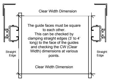
There are many ways to verify that the steel and guides are square to each other. This straight edge method is just one. We are concerned that the throat of the guide is square, so the end blocks do not wear unevenly.
