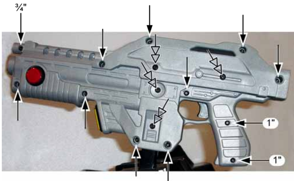
Figure 17. Gun Case Screws
