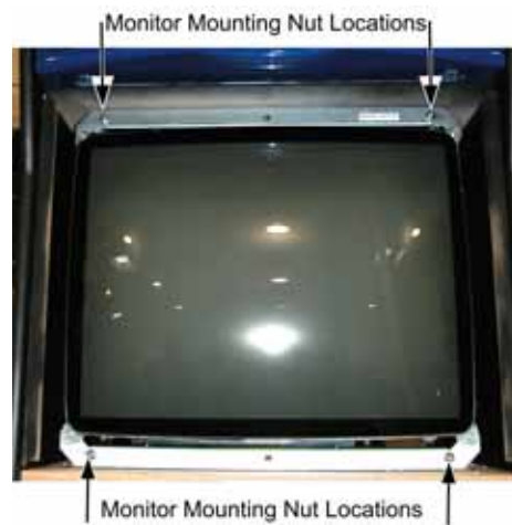
Figure 25. Monitor Mounting Nut Locations
