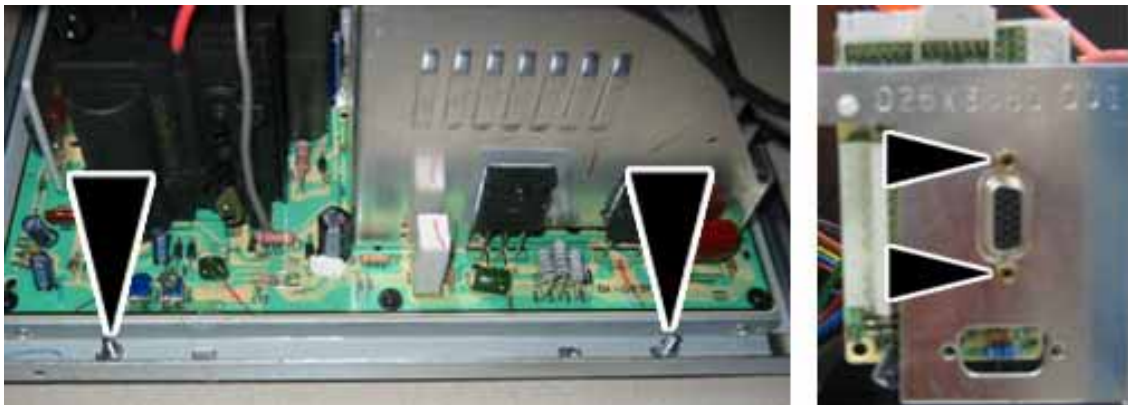
Figure 26. Removing the Monitor PCB Mounting Hardware
