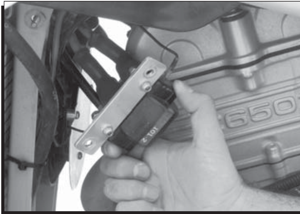
Figure 7 Removing the Factory Coil.
