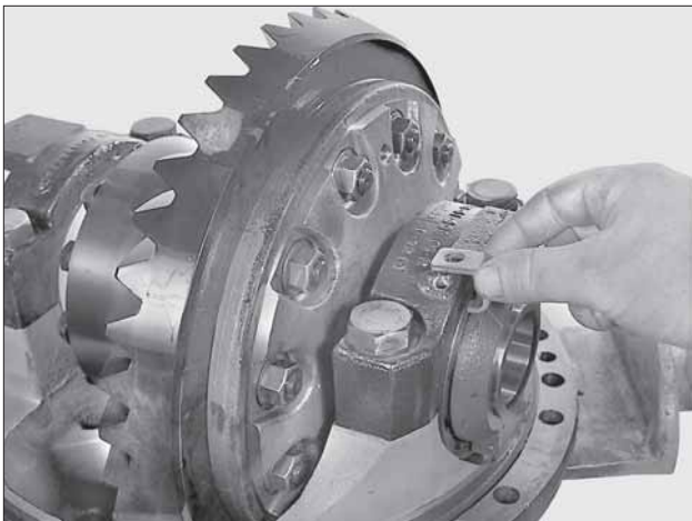
Figure 9 Remove (2) adjusting nut locks.
