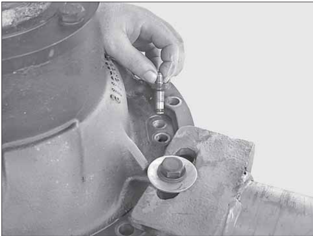
Figure 7 Remove tank and pressure port nipples.
