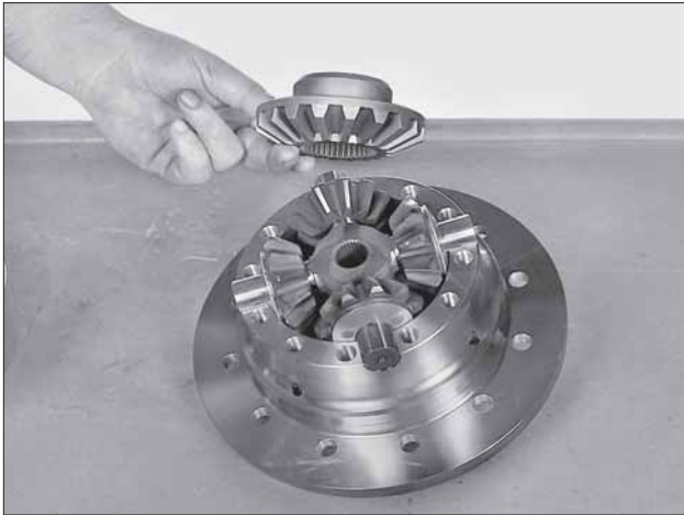
Figure 37 Position standard side gear on pinion and cross assembly.
