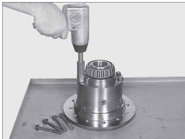
Figure 28 Remove (16) case cap half to clutch housing bolts and washers.
