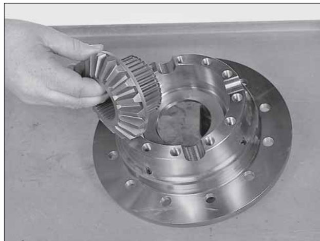
Figure 35 Install clutch side gear.
