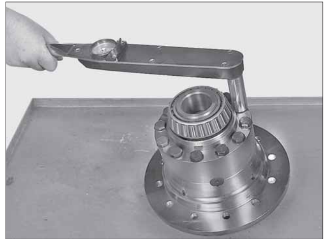
Figure 40 Install (16) case bolts and install with washers. Tighten to 71-88 Nm [52-65 LBF/FT].
