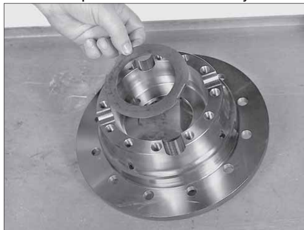
Figure 34 Position side gear thrust washer in clutch housing.
