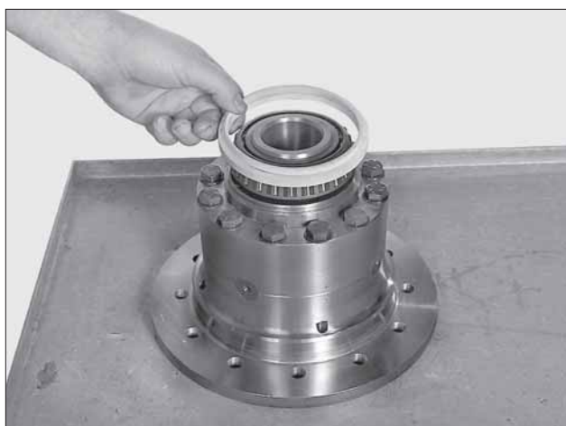
Figure 27 Remove differential case seal. Using appropriate puller remove bearing cone if replacement is required.
