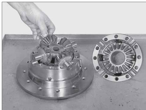
Figure 29 Separate case halves.
