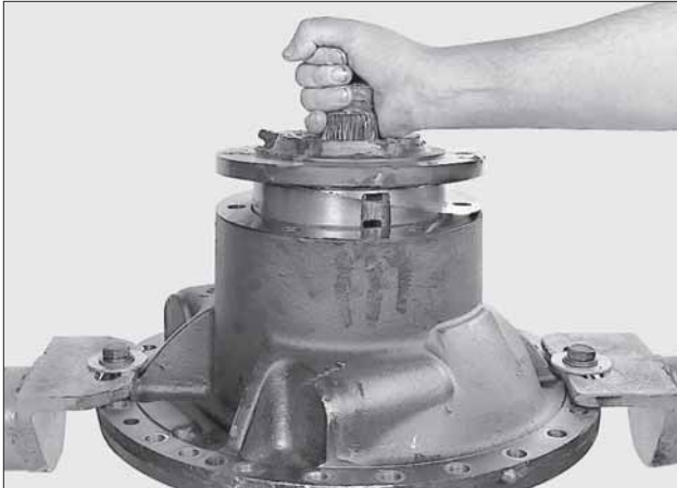
Figure 69 Press pinion into bearing retainer assembly. Install pinion and retainer assembly in carrier housing. NOTE: Line up oil holes in retainer and carrier housing.
