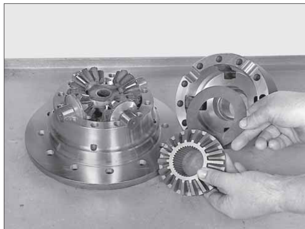
Figure 30 Remove side gear and thrust washer from case cap half.
