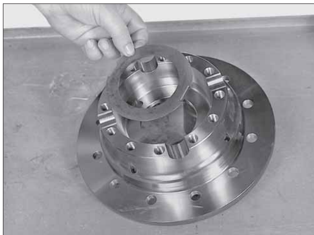
Figure 33 Remove clutch side gear thrust washer.
