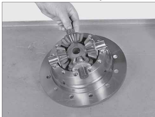
Figure 36 Assemble differential cross, (4) pinions and (4) thrust washers and install as an assembly.
