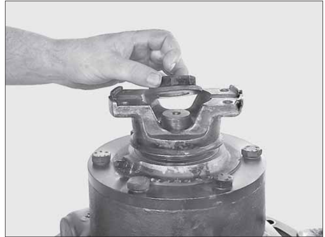
Figure 71 Install flange and flange o-ring. Apply Loctite 270 or equivalent to threads and install flange nut. Tighten to 600-800 Nm [443-590 LBF/FT].
