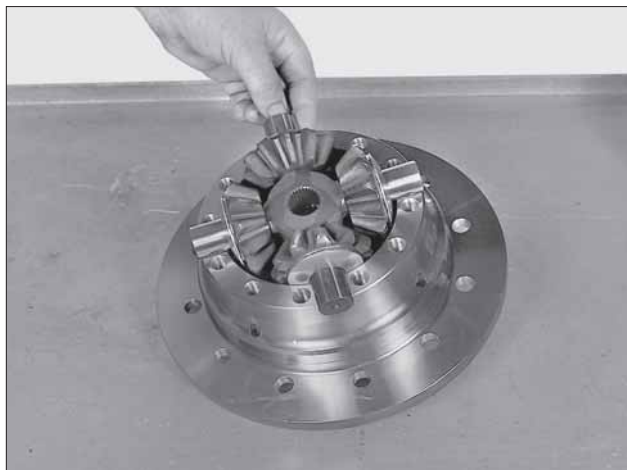
Figure 31 Remove differential cross, pinions and thrust washers from clutch housing.
