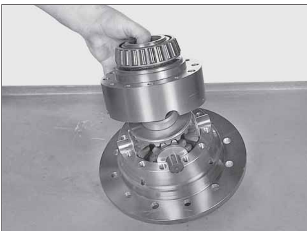
Figure 39 Using appropriate driver install bearing cone on case cap half. Position case cap half and bearing on clutch housing. NOTE: Be sure to match up alignment marks made during disassembly.
