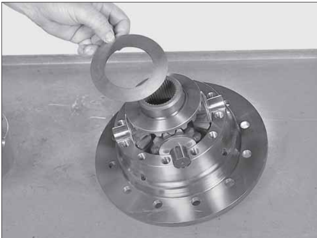
Figure 38 Place side gear thrust washer on side gear.
