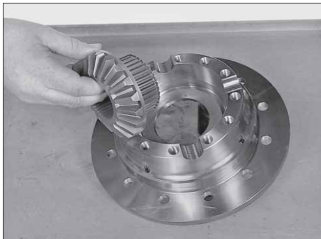
Figure 32 Remove clutch side gear.
