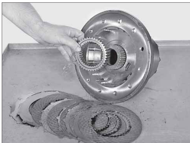
Figure 26 Remove clutch driver.
