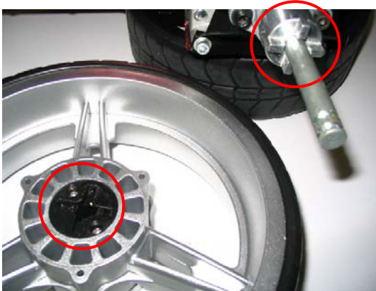
Align the four slots on the wheel with those on the drive dog teeth.
