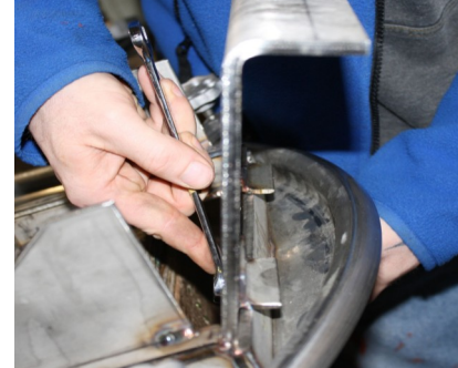
30. Insert 1/4" bolt through top of trap door. Using 7/16" wrenches, tighten lock nut, with 1-2 threads showing.
