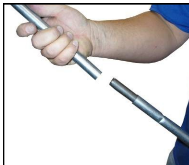
35. Assemble stir rod by inserting upset end over straight end and push together.
