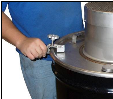
31. Rotate clamps into position and tighten by turning knob.
