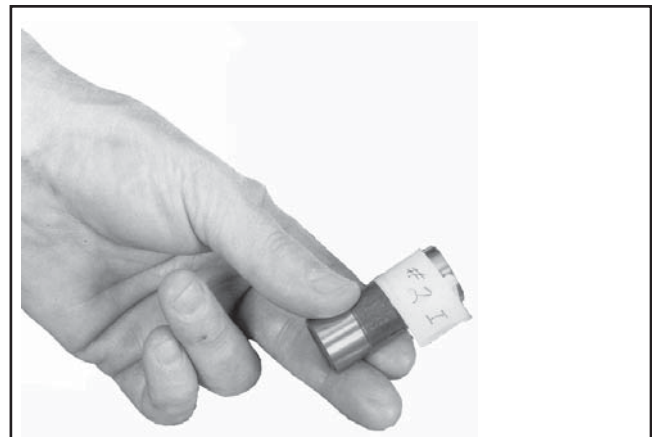
Figure 8-53. Mark the Lifters By Location.
