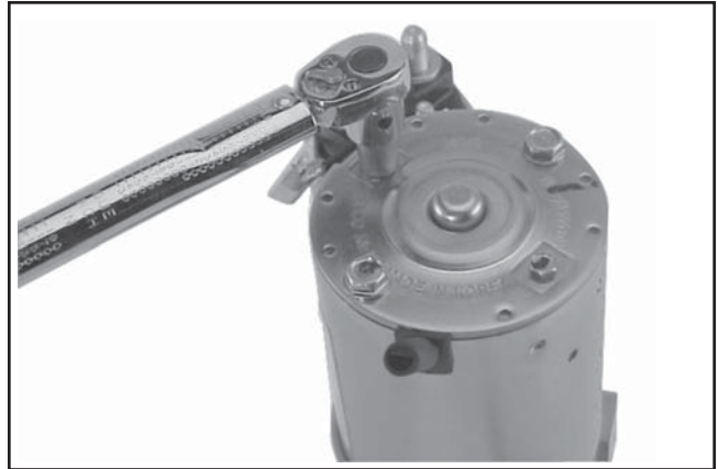
Figure 7-35. Torquing Brush Holder Screws.
