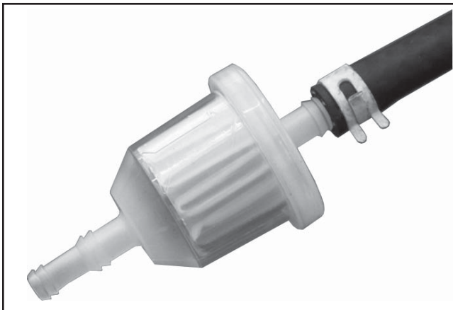
Figure 5-19. In-Line Fuel Filter.
