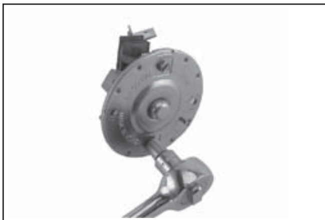
Figure 7-22. Removing Brush Holder.
