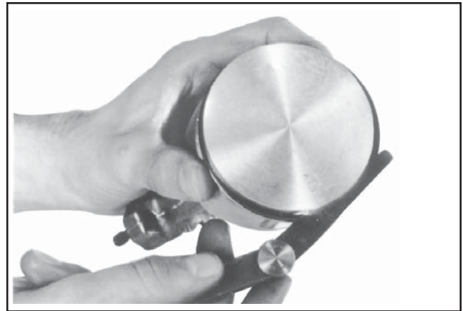
Figure 9-10. Measuring Piston Ring Side Clearance.
