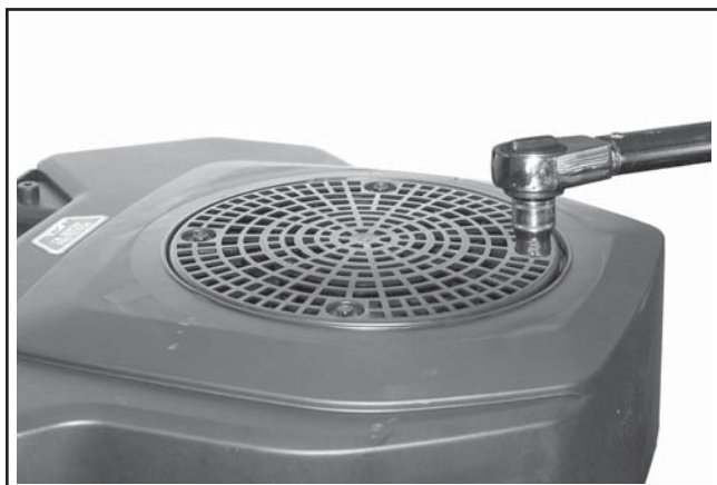
Figure 10-65. Torque Plastic Grass Screen Hex Screws.
