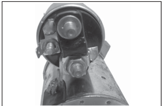
Figure 7-36. Positive (+) Brush Lead Connection.
