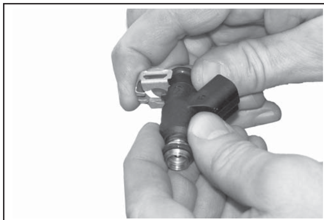
Figure 10-44. Install Fuel Injector Retaining Clip.
