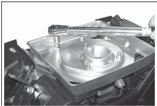
Figure 10-88. Torquing Base Mounting Nuts.
