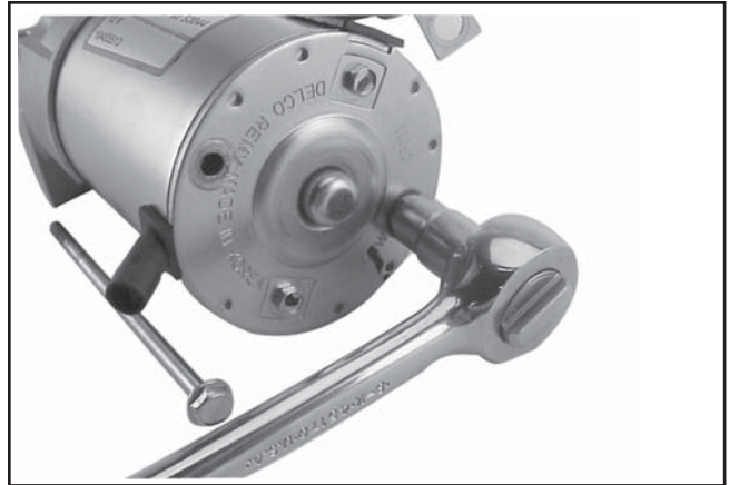
Figure 7-12. Removing Thru Bolts.
