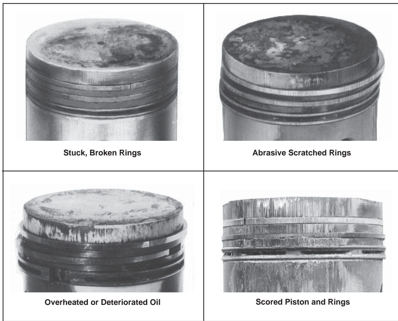
Figure 9-8. Common Types of Piston Damage.
