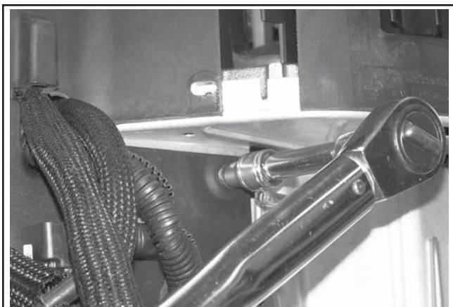
Figure 10-57. Tightening Short Screws for Outer Baffles.
