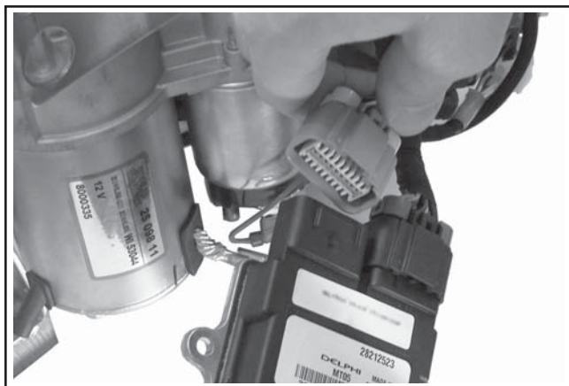
Figure 8-23. Disconnect ECU Electrical Connectors.
