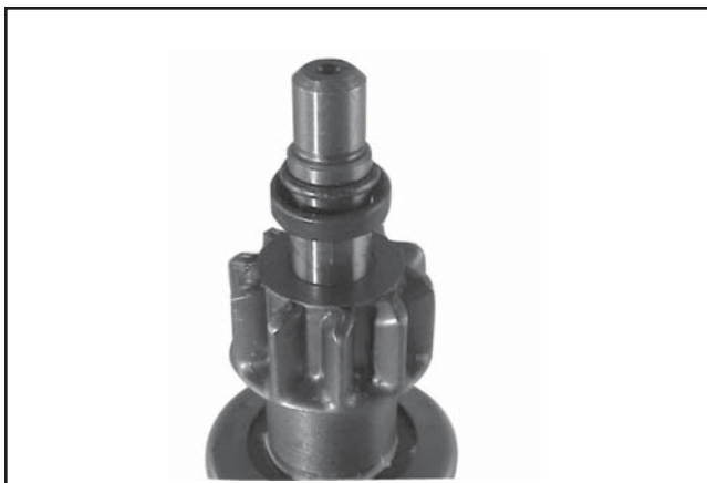
Figure 7-17. Retaining Ring Detail.
