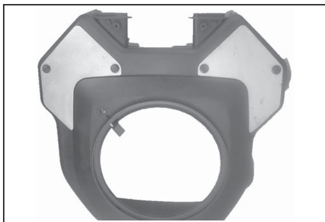
Figure 4-10. Cleanout Kit Installed on Blower Housing.
