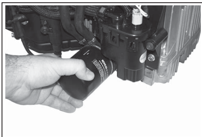
Figure 8-4. Removing Oil Filter.
