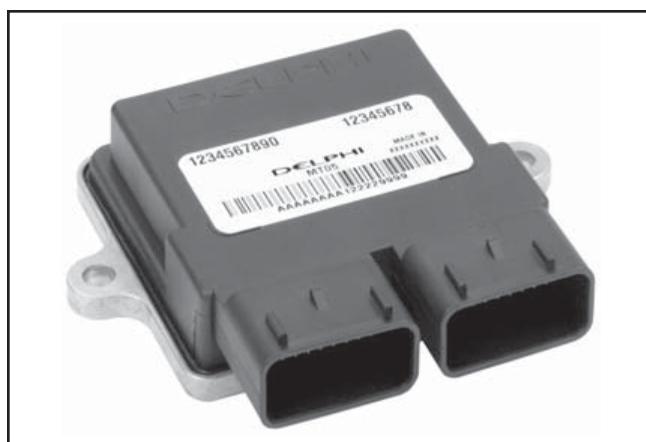
Figure 5-1. Electronic Control Unit (ECU).
