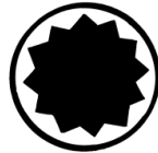
Opel Head Bolt Tops: "Serrated" (NOT Torx!)
