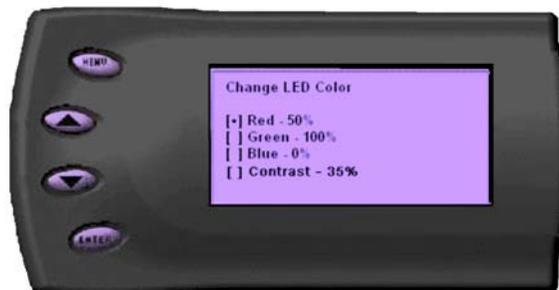
Depending on the color you select, a screen similar to the photo to the right will appear. Use the arrow keys to adjust the percentage shown on the screen. Once the desired color value has been reached, press [ENTER]. To return to the previous screen and abort the current change, press [MENU].
