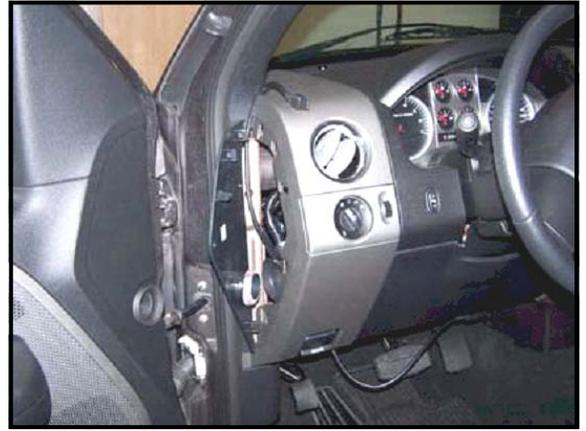
Feed roughly 8 to 10 inches of cable through the dashboard with one end of the cable protruding through the front of the Pod. With the Pod secure, attach the Gryphon™ to the cable.
