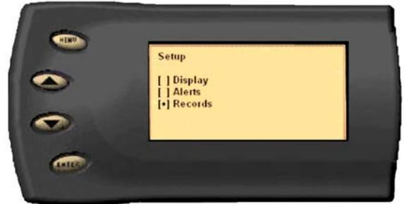
From this screen, you can view all of the current high values that have been recorded. The arrow on the bottom right corner indicates that there are more parameters than the display can show. Use the arrow keys to scroll through the list. To reset all of the records, highlight **Clear All** and press [ENTER]. To reset a single record, highlight the desired parameter and press [ENTER]. Press [MENU] to exit out of this list.
