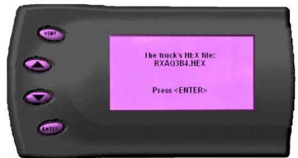
\*If no hex code is shown, disconnect from the OBDII plug and reconnect it after 5 seconds. When you come to the screen again, the code should be available.
