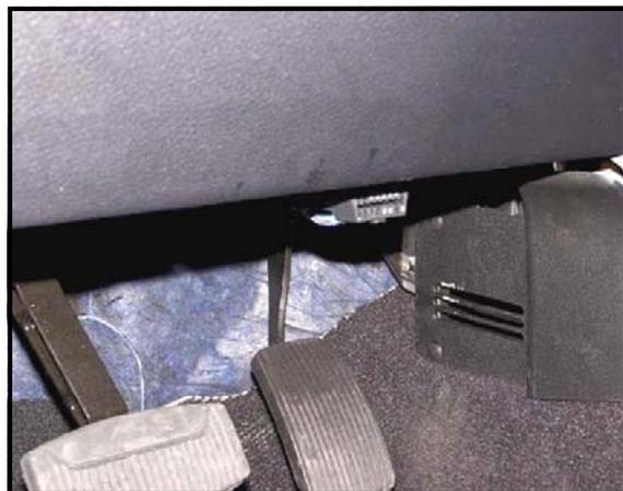
With the driver's side door open, remove the access panel on the left side of the dashboard.
