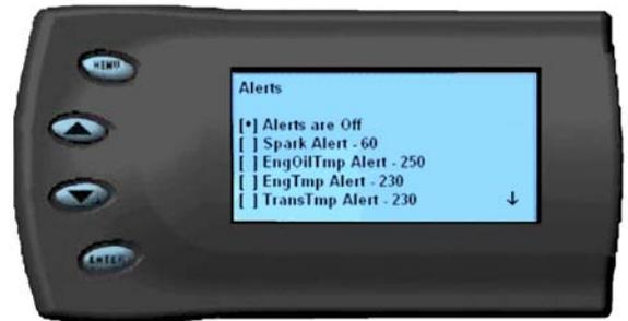
To change the value of a specific alert, select the PID you would like to change and press [ENTER]. A screen similar to the photo to the left will appear. Use the arrow keys to reach the desired value. Press [ENTER] to save the current alert. Press [MENU] to return to the previous screen.
