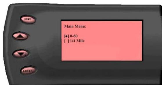
For the 0-60 MPH run, press the accelerator pedal and the test will automatically begin. As you drive, the screen will display your current speed. The test will stop automatically and your time will be displayed on the screen.
