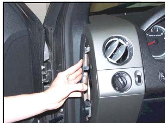
Pull the end of the OBDII cable outwards. Snake it up to the A-pillar of the vehicle and replace the access panel. The cable should be protruding from the dashboard up along the A-pillar and be able to move freely when pulled.
