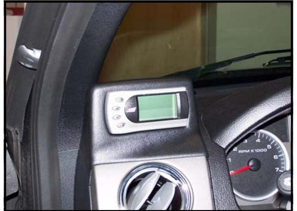
The Gryphon™ logo will display followed by a disclaimer. After you agree to the disclaimer by pressing [ENTER], the following screen will be displayed. This is the HEX code of the truck to which the Gryphon™ is currently connected.\*
