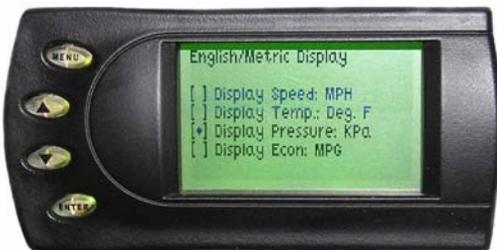
Select the display units you would like to change. Here, **Pressure** has been selected and was changed to kilo/Pascals (Kpa) by pressing [ENTER]. Each time you press [ENTER] on a selection, the display toggles between English and metric units.
