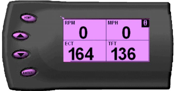
From this display, press [MENU] to select and use other features of the Gryphon™. The display backlight can also be controlled from this display using the [UP] and [DOWN] arrow keys.
