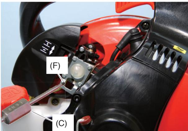
1. Start engine and warm it up alternating engine speed between WOT and idle every 10 seconds for 1 minute.
