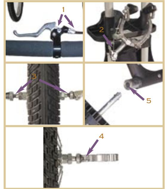
Replace the brake pads when the grooves become worn away. Check all bolts are tight and springs are secure for rear foot brake.
