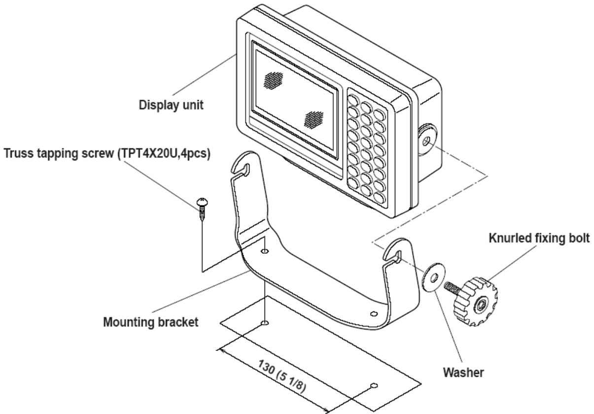
Figure 4.1 Fitting detail of KGP-920 in table mounting mode
