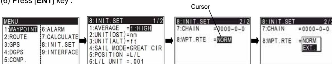
A small E is displayed at the end of the way point identifier to show KGP-920 is in external mode.
