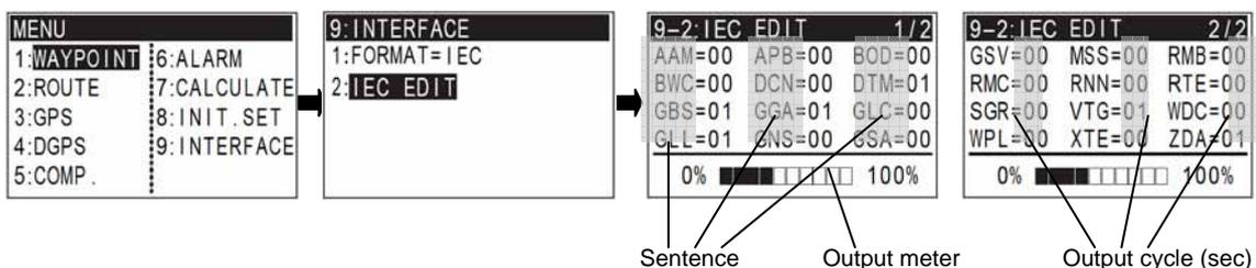
**NOTE:** Set the output cycle for the required sentence only and set the unused data to "00". The output meter indicates the ratio of total data amount (of selected sentence) to the data transmission capacity (about 10% per scale). Do not maximize at 100% or poor performance may result.
