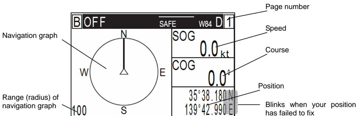
**NOTE:** The navigation graph shows your boat position and the relative bearing.
