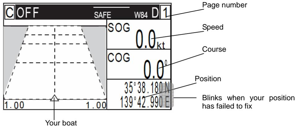
NAV3 screen shows a 3-dimensional view indicating the distance, course, cross track error, and deviation from the waypoint. The boat icon does not move in OFF mode.
