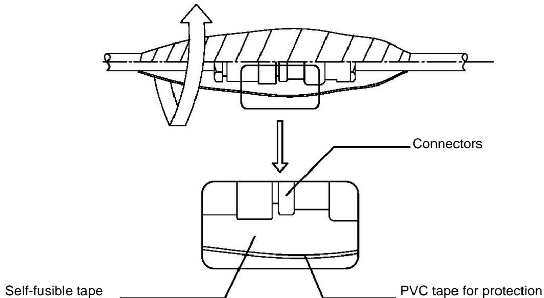
**Figure. 4.5 Processing on the coax cable jointing section**
