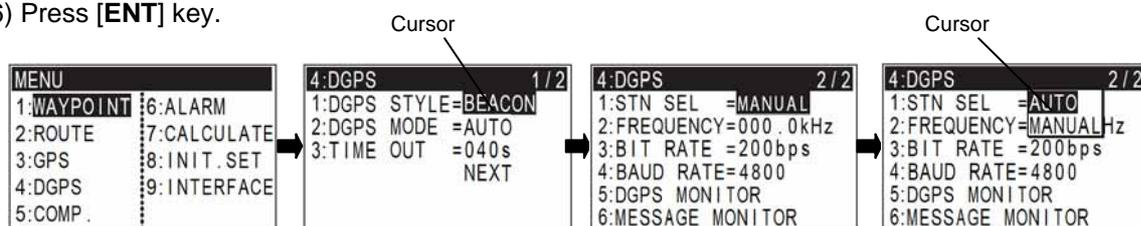
**(Selecting a station in the manual mode)****Internal beacon receiver system**
