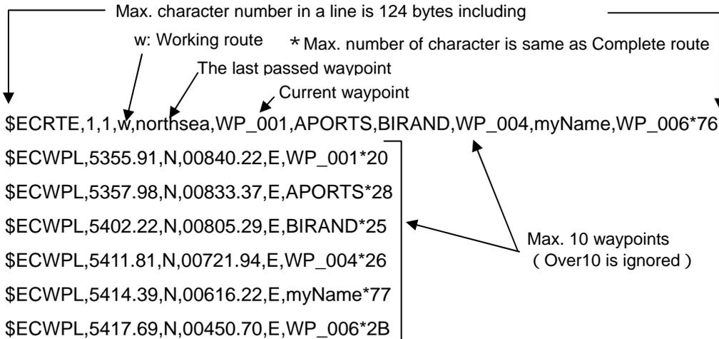
Working route has priority and route navigation by Working route automatically begins by reception of working route data. It is updated every time Working route data is received.
