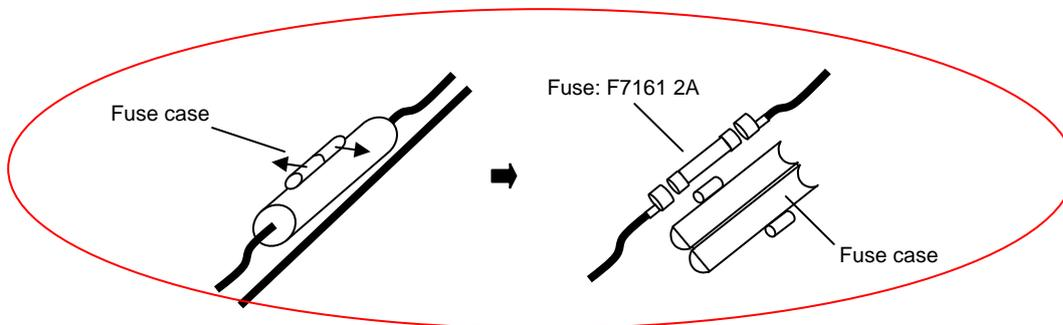
Figure 10.1 Replacing the fuse
