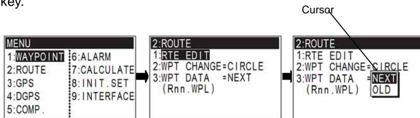
**8.6.5 Selecting an output data format of DATA 2 port .** Initial setup: Extension data port
