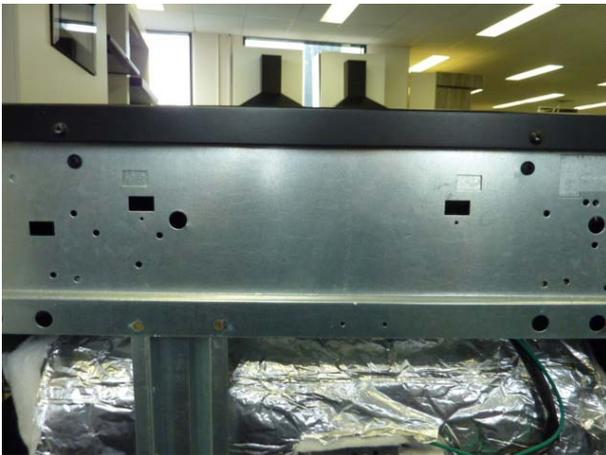
REMOVE 4 X SCREWS THAT HOLD THE ELEMENT BASE TRAY IN PLACE
