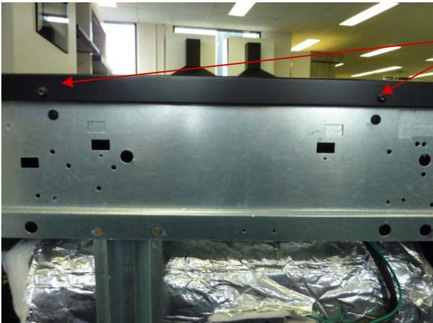
REMOVE 4 X SCREWS IN SIDE OF HOTPLATE (2 EACH SIDE )
