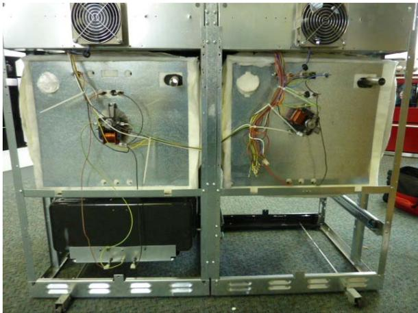
REMOVE COVERING PLATE AT THE BACK OF THE OVEN CAVITY
