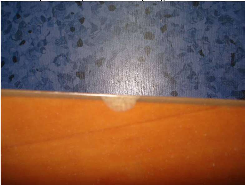
Figure 2 – Trailing Edge Chip
