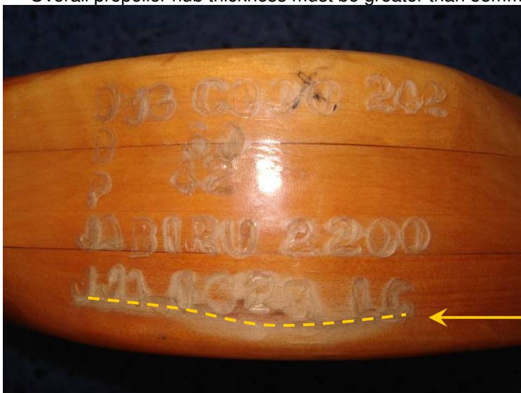
Figure 4 – Hub Compression Cracking
