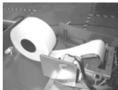
Figure 6-7. A new roll of paper installed on the Printer.
