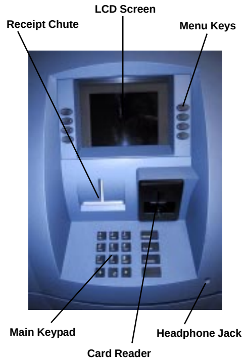
Figure 2-2, Control Panel Interface.
