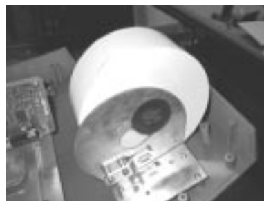
Figure 6-5A. Placing the paper roll and spool on the paper bracket.
