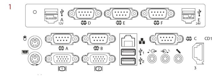
The RS232 ports are labeled A, B, C, D, E, F and ports C-F have power indication icons. Powered USB ports are designated A-E with appropriate power indication. The Cash drawer port is designated CD1 and also has the number 3 in close proximity.
