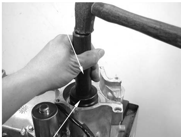
Bearing Outer Driver, 42x47mm Pilot, 20mm
