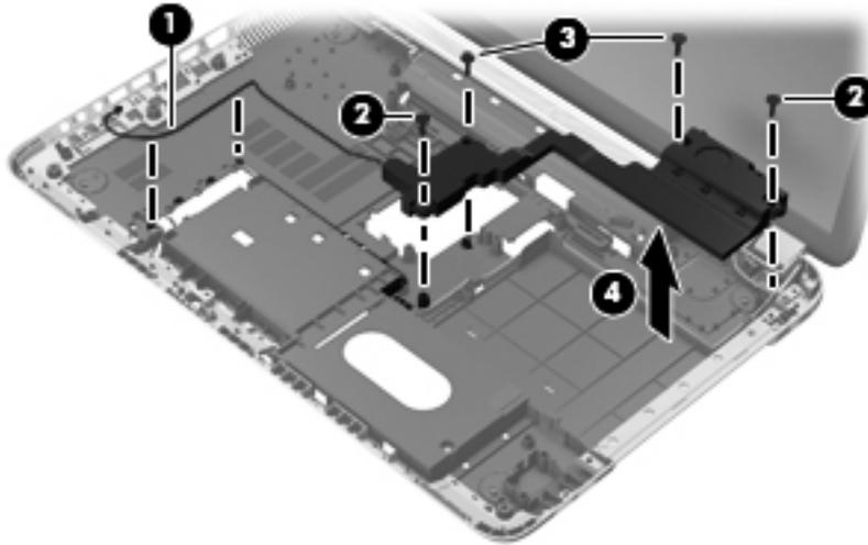
Reverse this procedure to install the subwoofer and cables.
