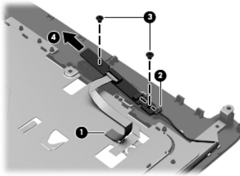
Reverse this procedure to install the power button board.
