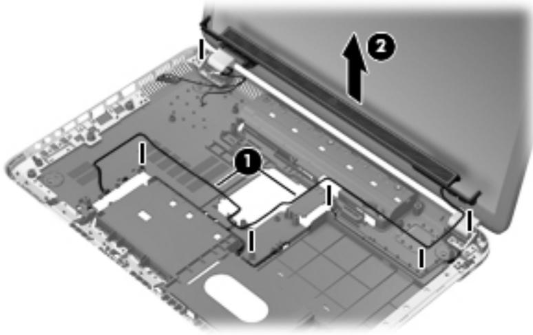
Reverse this procedure to install the rear speakers and cables.
