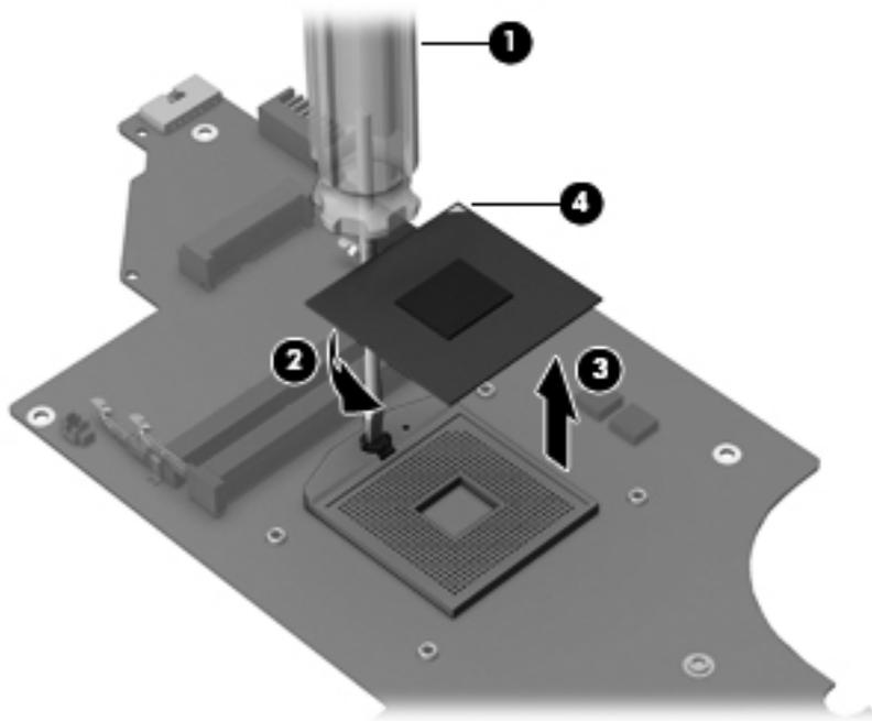
Reverse this procedure to install the processor.
