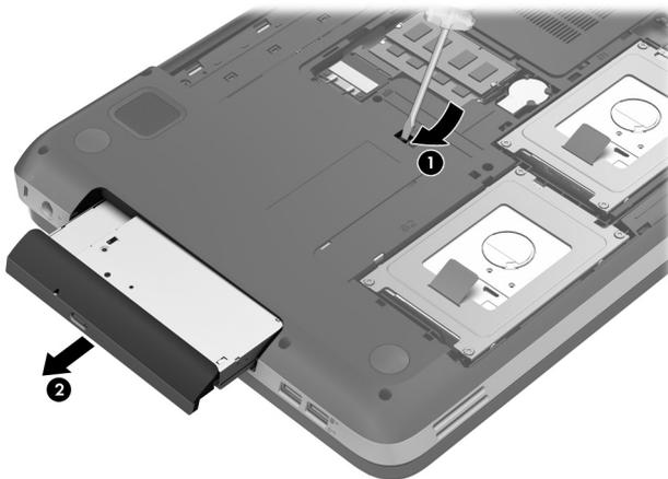
5. Push on the hard drive bracket **(1)** to release the optical drive.
