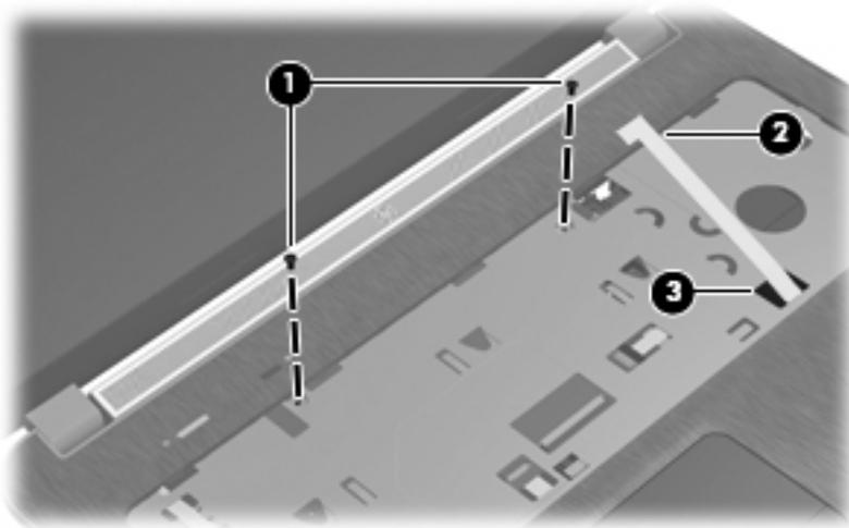
9. Lift the rear edge of the top cover (1) until the left and right sides disengage from the base enclosure.
