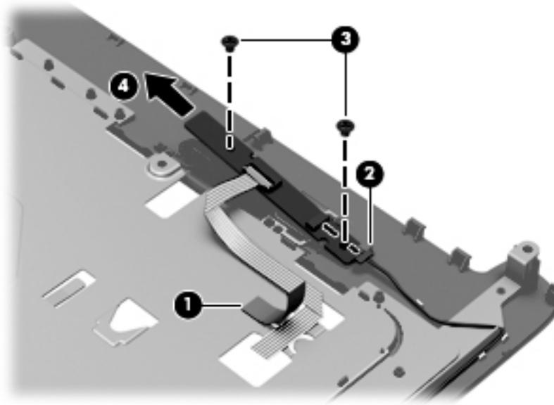
5. Remove the display lid switch board and cable.
