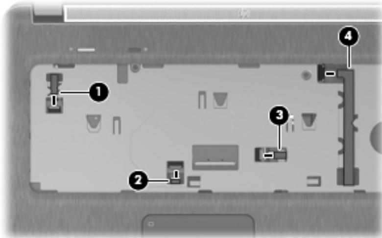
8. Remove the two Phillips PM2.5×5.0 screws that secure the top cover to the computer.
