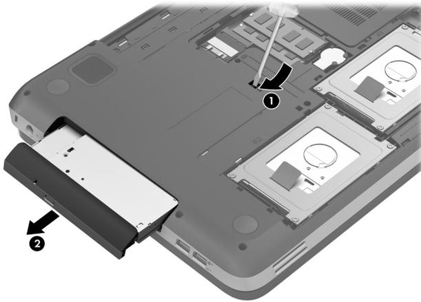
7. If it is necessary to replace the optical drive bracket, position the optical drive with the rear panel toward you.
