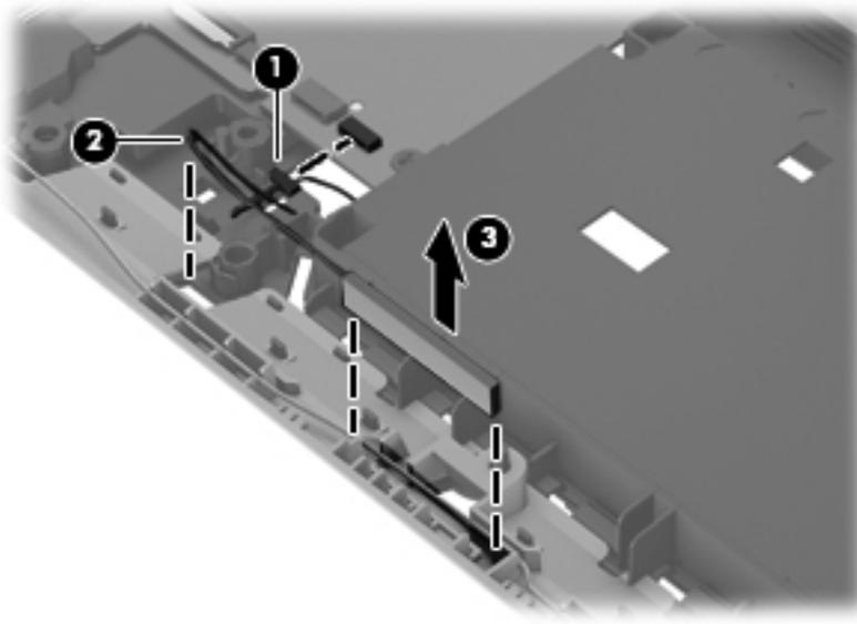
4. Remove the Bluetooth module and cable.
