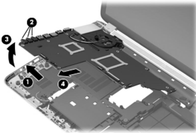
Reverse this procedure to install the system board.
