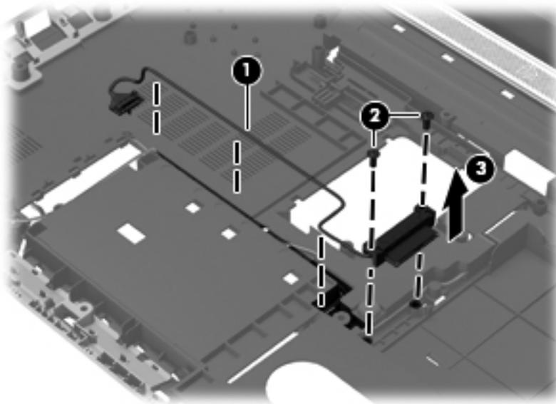
Reverse this procedure to install the optical drive cable.
