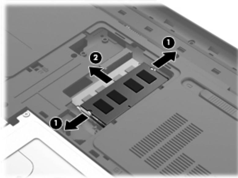
Reverse this procedure to install a memory module.
