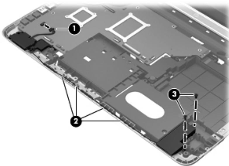
4. Rotate the front left speaker **(1)** clockwise to release it from under the system board.
