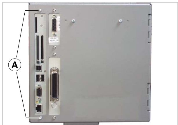
[183] Fastening of the CPU board to the back casing.
