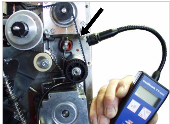
[67] Checking the belt tension with a frequency meter.
