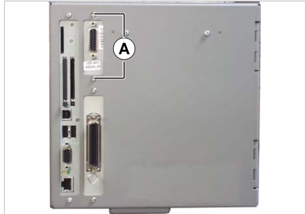
[178] Fastening (A) of the USI board to the back casing.
