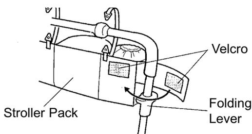
1. Wrap the side velcro straps tightly around the handle tube above the Folding Lever.
