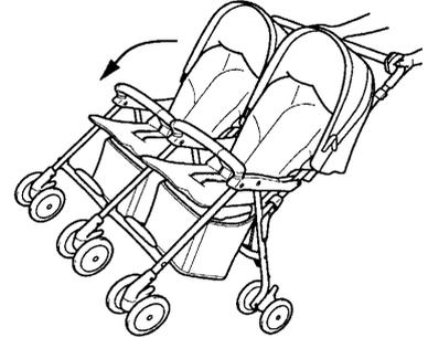
3. Lift up the handle bar and snap it away from you. It will open and automatically lock into position.
