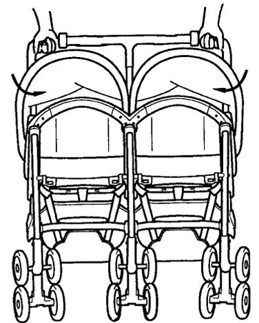
8. Latch the folding latch to hold the stroller together.
