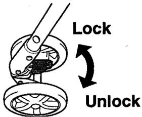
To lock swivels, lift all swivel lock levers **up**.
