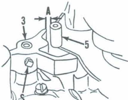
Fig. M7-8—Cluster lever (3) must be adjusted on throttle shaft on some early models. Refer to text.
