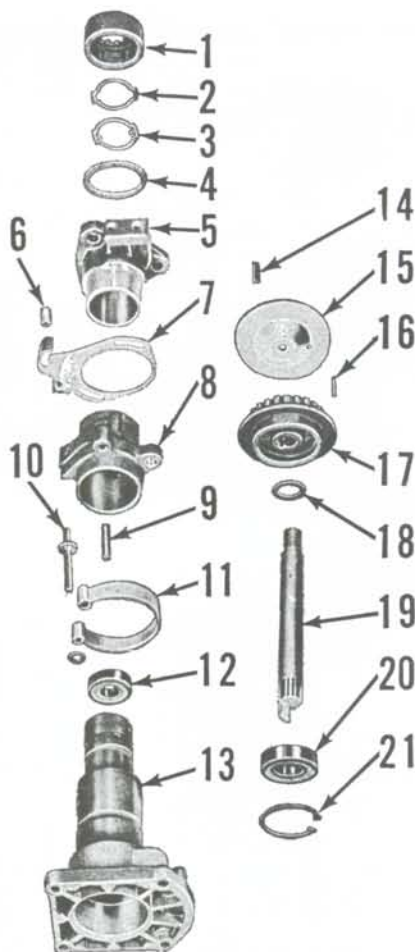
Fig. M7-21—Exploded view of distributor mounting bracket and drive mechanism used on some models. Others, including magnetos, are similar.
