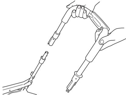
7. Insert long grey tabs into grey plastic slots on the stroller frame. Grey tabs must be fully inserted into the slots in order to fold the stroller.
