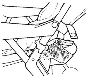
2. Loop the rear straps of the basket through the waist belt and snap together.
