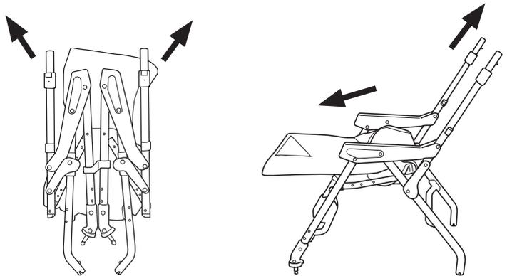
6. Insert stroller handle into frame by pressing chrome buttons into the back of the stroller frame.
