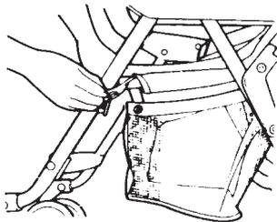
1. Loop the front strap of the basket over the seat frame and snap together.
