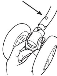
4. Insert the leg into the wheel assembly until the small chrome pin locks into the opening.
