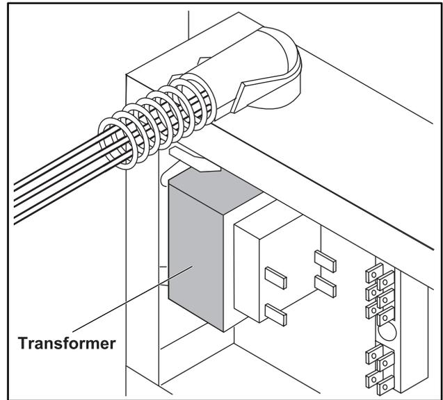
**Figure 5. 240/208 Step Down Transformer**
