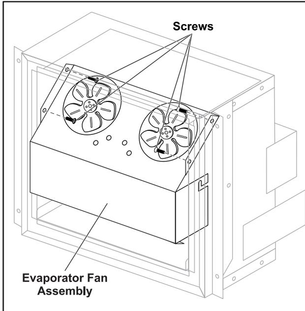
**Figure 12. Evaporator Fan assembly**
