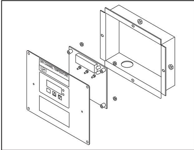
**Figure 3. Exploded View of Relay Box Internal Components**
