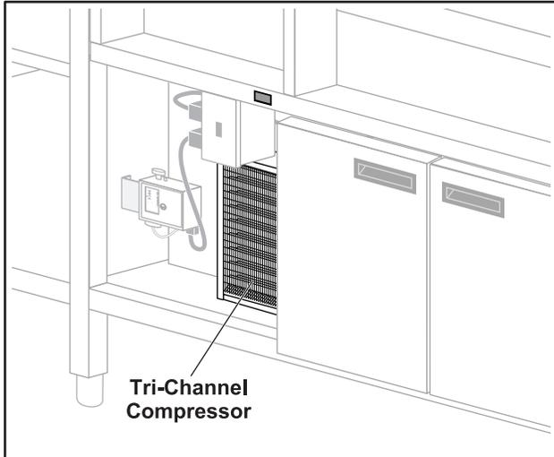
**Figure 10. Compressor Assembly**
