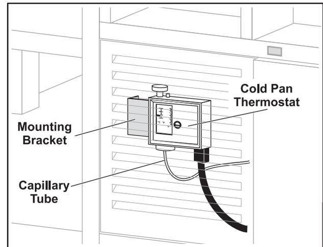
**Figure 9. Location of Tri-Channel Cold Pan Thermostat**
