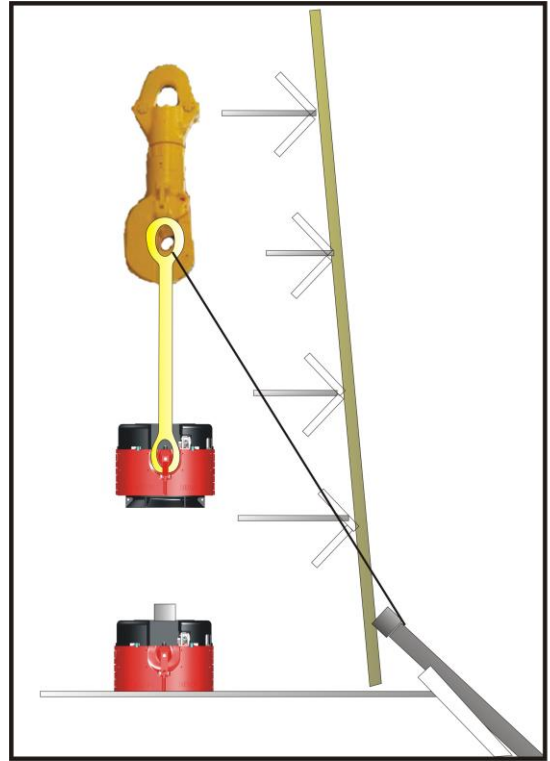
Figure 2-7. Standard Derrick Installation
