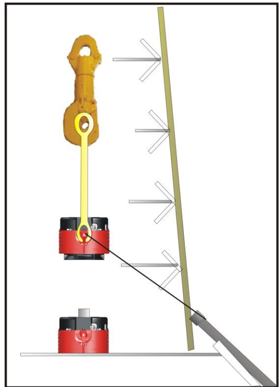
Figure 2-8. Jackknife Derrick Installation
